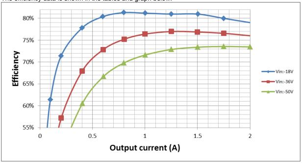
$V_{in}$ =-18 $V_{DC}$
