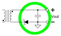
Figure 1. Diode that was replaced w located such that its anode is connected to GND; otherwise, additional circuitry would have been required.
