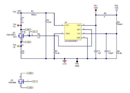
Figure 5 PMP11216 Schematic
