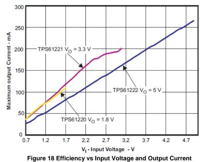
6.2.1 Efficiency vs Input Voltage and Output Current
