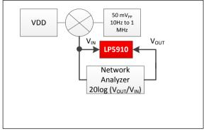
Figure 9 PSRR Test Setup
