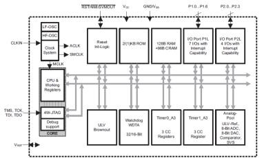
Figure 4 Functional Block Diagram, MSP430C092PW, and MSP430C091PW
