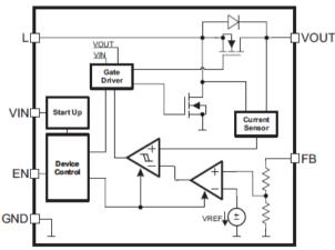
Figure 2 TPS61221 Functional Block Diagram
