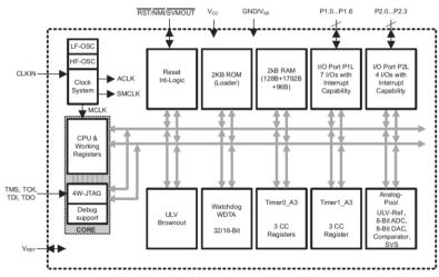
Figure 3 Functional Block Diagram, MSP430L092PW
