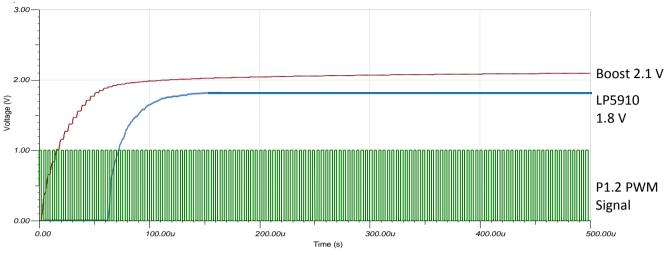
Figure 7 Boost Circuitry Output Voltage
