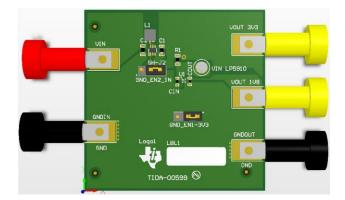
TIDUA73 - September 2015 LP5910 and TPS61221 as a Power Reference Design for Ultra-Low Voltage MSP430X09X Companion Devices
