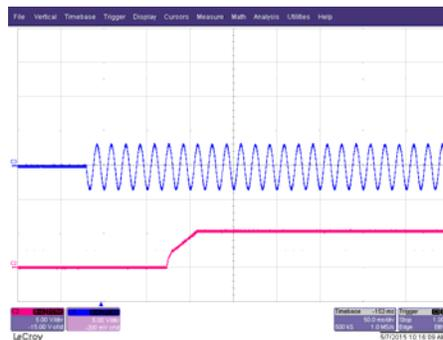
Figure 9 Output voltage start 230Vac, Full Load
