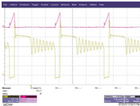
Figure 14 Primary switching voltage and current at 230Vac and full load
