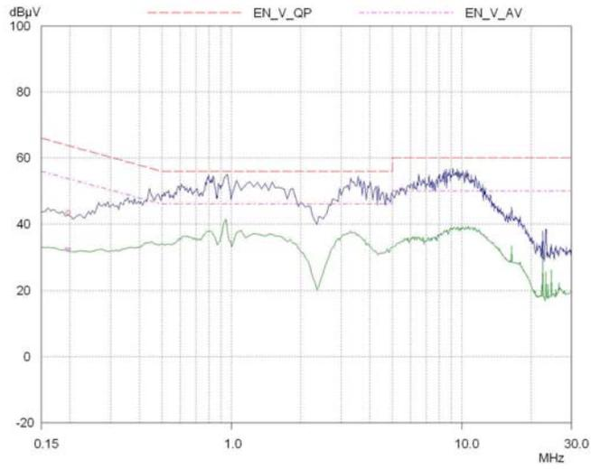
Figure 17 Conducted Emissions at 115Vac and full load with load grounded
