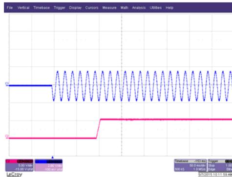
Figure 8 Output voltage start, 115VAc, No Load load
