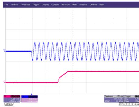
Figure 7 Output voltage start 115Vac, Full Load
