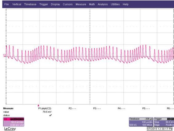
Figure 5 5V ripple with both outputs at full load
