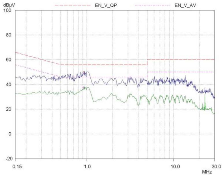
Figure 16 Conducted Emissions at 230Vac and full load with load ungrounded
