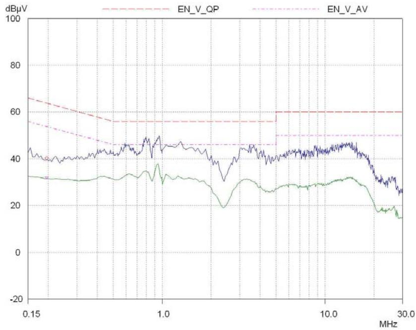
Figure 15 Conducted Emissions at 115Vac and full load with load ungrounded
