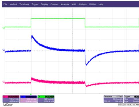
Figure 11 Step Load 5V(0.1A to 0.5A) 12V(0.5A)
