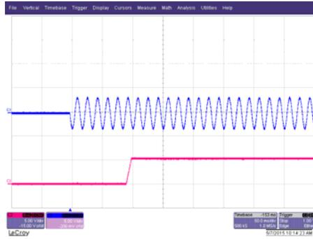
Figure 10 Output voltage start 230Vac, No Load
