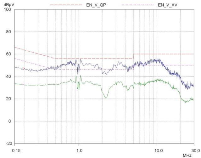
Figure 18 Conducted Emissions at 115Vac and full load with load grounded
