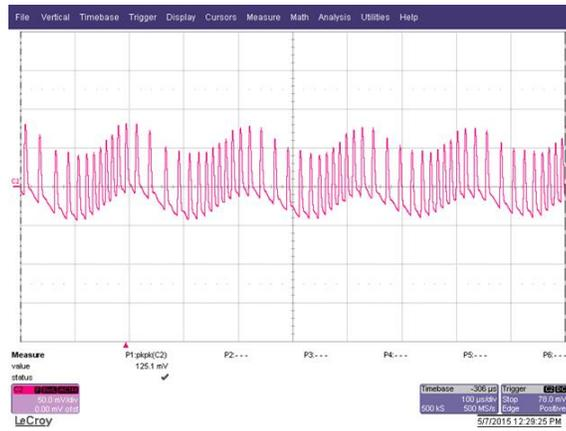
Figure 4 12V ripple with both outputs at full load
