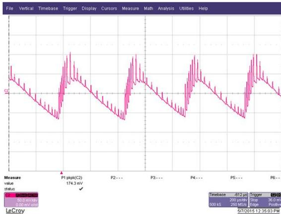
Figure 6 Worst case ripple for 12V rail (12V at no load and 5V at full load)
