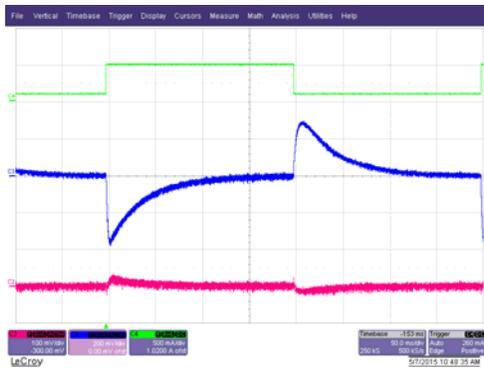
Figure 12 Step Load 12V(0.1A to 0.5A) 5V(0.5A)
