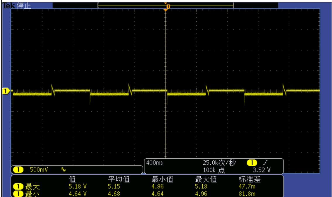
Vin:230Vac test condition: 0%-100% of full load, 0.4A/us, 500ms cycle, 100cm cable
