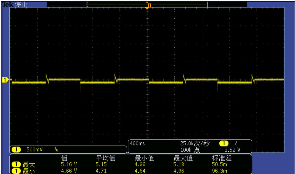
Vin:115Vac test condition: 0%-100% of full load, 0.4A/us, 500ms cycle, 100cm cable
