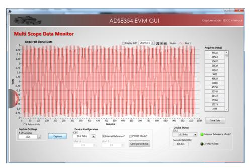
Figure 49. 16-Bit ADS8354 at 60 kHz
