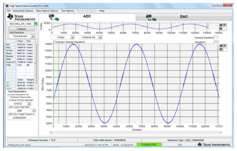
Figure 34. ADC3441—AC Input With Resistor Divider at 400 Hz
