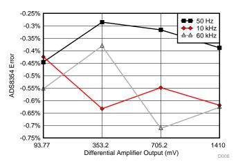
Figure 52. Differential Amp Output versus 16-Bit ADC Error
