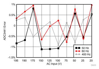
Figure 40. THS4521—AC Input vs ADC Error
