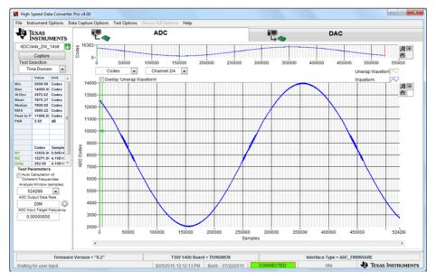
Figure 32. ADC3441—AC Input With Resistor Divider at 50 Hz
