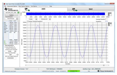
Figure 36. ADC3441—Function Generator Input at 1 MHz
