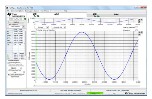
Figure 33. ADC3441—AC Input With Resistor Divider at 60 Hz
