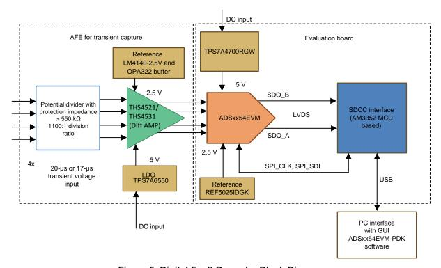
Figure 5. Digital Fault Recorder Block Diagram
