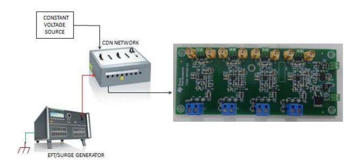
Figure 53. Surge Setup for AFE Used in TR and DFR
