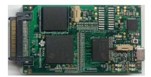
Figure 16. SDCC Card of ADSxx54 Board
