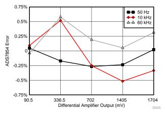
Figure 51. Differential Amp Output versus 14-Bit ADC Error
