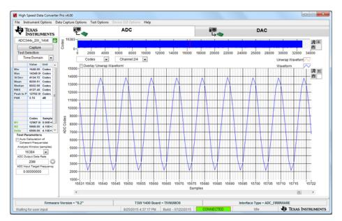
Figure 37. ADC3441—Function Generator Input at 2 MHz
