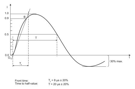
Figure 2. Waveform of Short-Circuit Current (8/20 μs)
