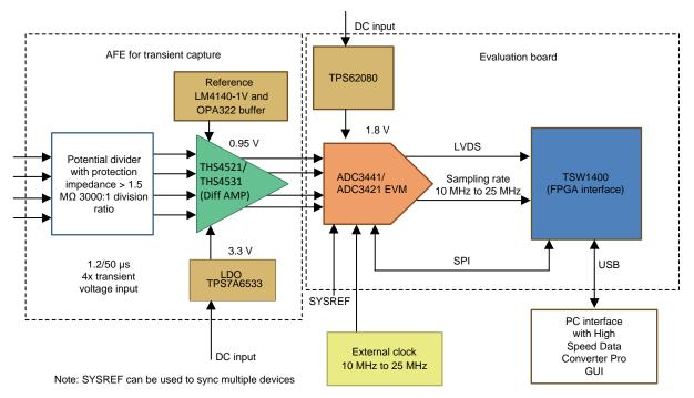
Figure 4. Transient Recorder Block Diagram
