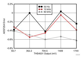
Figure 50. Differential Amp Output versus 12-Bit ADC Error
