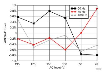
Figure 39. THS4531—AC Input vs ADC Error
