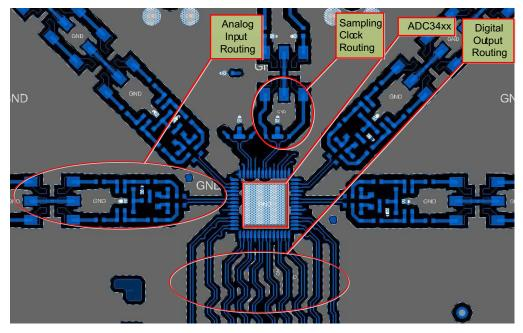
Figure 25. Typical Layout of ADC344x Board
