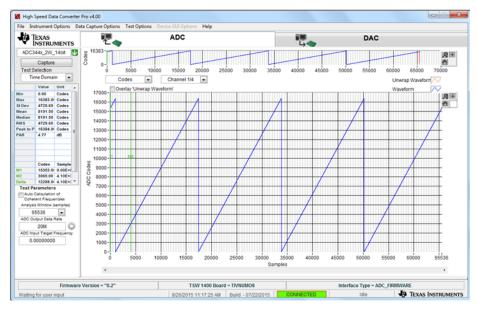
Figure 23. Self-Test for ADC3441
