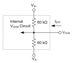
Figure 10. Circuit for V<sub>OCM</sub> Configuration
