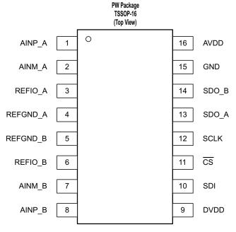
Figure 7. ADS7853 Pin Configuration
