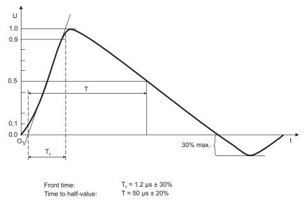
Figure 1. Waveform of Open-Circuit Voltage (1.2/50 μs)
