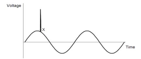
Figure 3. Impulsive Transient Showing Point X
