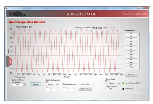
Figure 42. 12-Bit ADS7254 at 10 kHz
