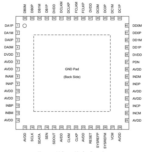
Figure 6. ADC3441 Pin Configuration
