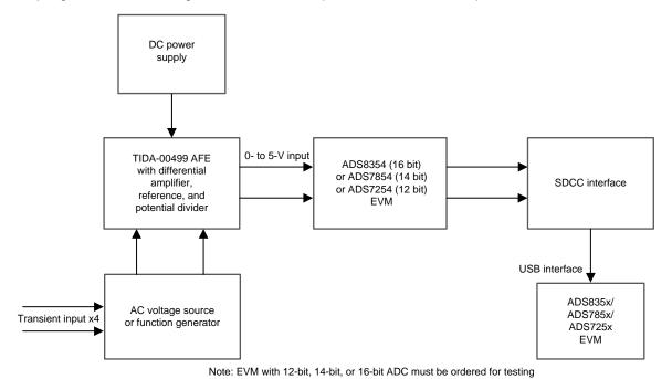
Figure 28. Test Setup Block Diagram for Digital Fault Recorder AFE Performance
