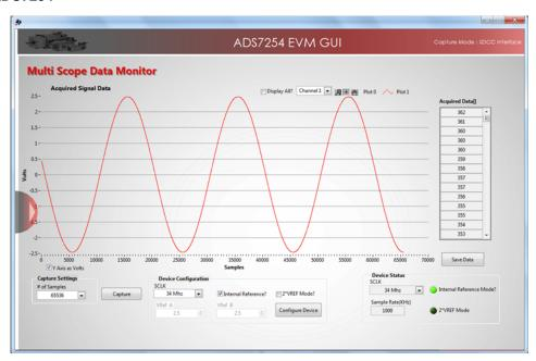
Figure 41. 12-Bit ADS7254 at 50 Hz
