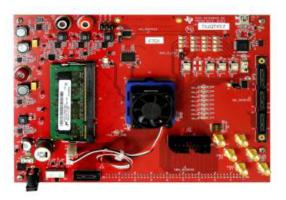
Figure 14. Top View of TSW1400EVM Circuit Board
