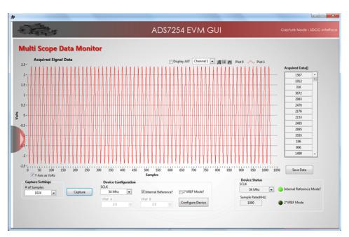
Figure 43. 12-Bit ADS7254 at 60 kHz
