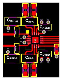
Figure 24. Recommended Layout for SAR ADC ADSXX53 Family
