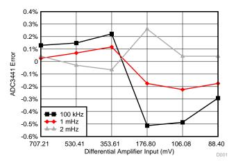
Figure 38. HF Input (mV) vs ADC Error
