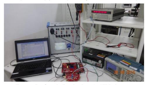
Figure 27. Test Setup for Transient Recorder AFE Performance
