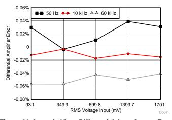
Figure 30. Input (mV) vs Differential Amp Output Error
