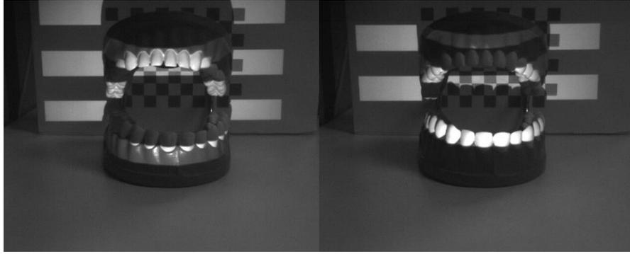
**Figure 40** Non-inverted and inverted horizontal Gray code pattern 3 capture
