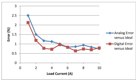
Figure 10: Analog and Digital Error vs Load Current, Battery Voltage = 400V
