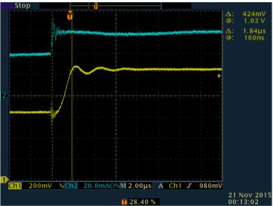
Figure 13: 4A to 6A Load Step Response Time
