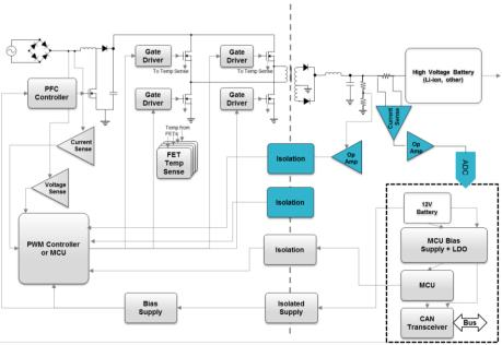
Figure 1: Complete Analog On-Board Charger System
