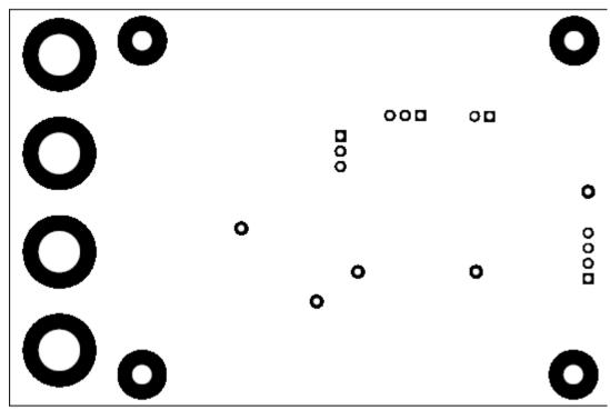
Figure 20: Bottom Solder Mask
