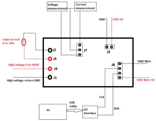
Figure 6: Test Set-up for TIDA-00456
