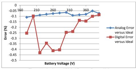
Figure 12: Analog and Digital Error vs Battery Voltage
