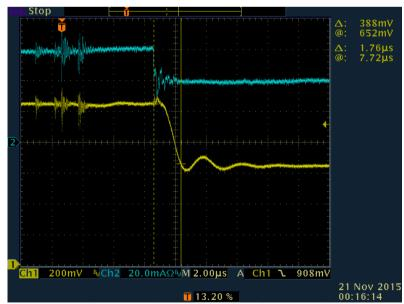
Figure 14: 6A to 4A Load Step Response Time
