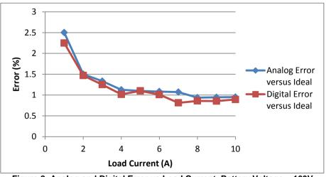
Figure 8: Analog and Digital Error vs Load Current, Battery Voltage = 160V
