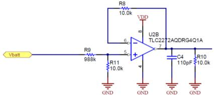
Figure 4: Battery Voltage Measurement Circuit
