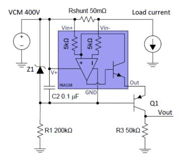
Figure 3: Schematic of INA138-Q1 in a High Common Mode Voltage Application
