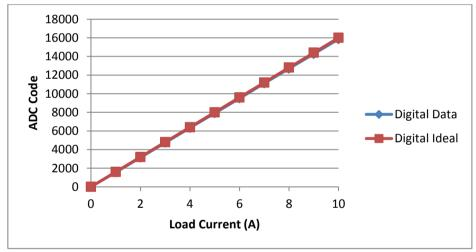
Figure 7: Digital Data and Digital Ideal versus Load Current, Battery Voltage = 160V
