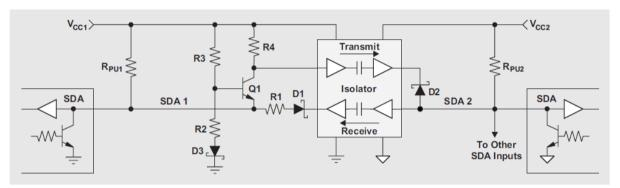
Figure 5: Bidirectional Communication with Digital Isolator
