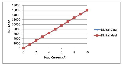
Figure 9: Digital Data and Digital Ideal versus Load Current, Battery Voltage = 400V
