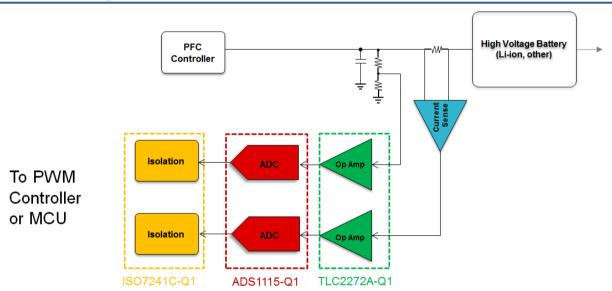
Figure 2: On-Board Charger Load Feedback Subsystem
