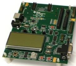
The CC2530-CC2592EM is an add-on module that can be plugged onto a SmartRF05EB. To run the example in this Quick Start Guide, two SmartRF05 boards are required to establish an RF link between the evaluation modules.
