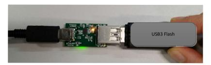
Figure 5. TIDA-00891 Test Setup example
