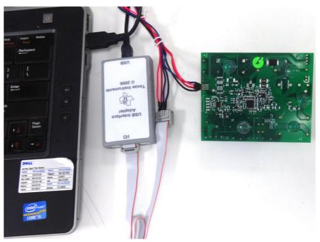
Figure 5. TIDA-00707 Setup for Programing UCD3138A
