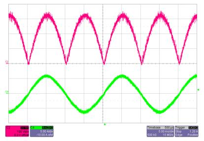
Figure 15. Input Voltage and Input Current at  $V_{INAC}$  = 230-V AC, Full Load
