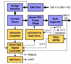
1-kW, Compact, 97.5% Efficiency, Digital PFC for AC/DC PSUs With eMeter
