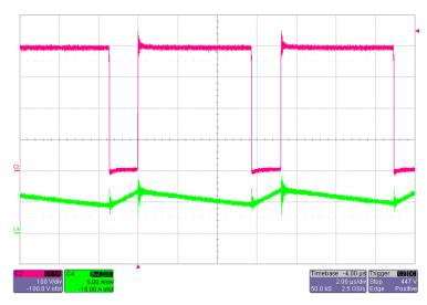
Figure 12. SW Node Waveform and MOSFET Current at  $V_{INAC}$  = 230-V AC, Full Load
