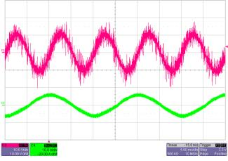
Figure 17. Output Voltage Ripple at  $V_{INAC}$  = 230 V, Full Load
