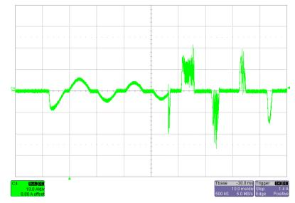
Figure 16. Output Voltage and Input Inrush Current at V<sub>INAC</sub> = 230 V, Full Load
