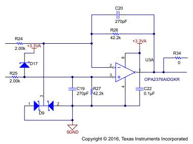
Figure 2. Amplifier Circuit for Current Sense Signal
