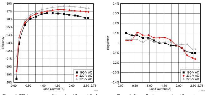
Figure 8. Efficiency versus Output Load Current (Iout)
