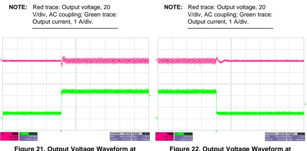
Figure 21. Output Voltage Waveform at V<sub>INAC</sub> = 230 V, Load Transient From 0.5 to 2.56 A Figure 22. Output Voltage Waveform at  $V_{INAC}$  = 230 V, Load Transient From 2.56 to 0.5 A
