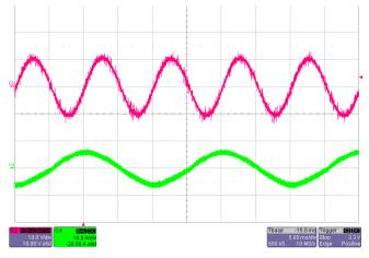
Figure 18. Output Voltage Ripple at V<sub>INAC</sub> = 230 V, Full Load, Only 50-Hz Component
