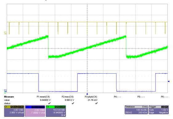
Figure 38. Droop Rate at 25°C With Exaggerated Hold Time
