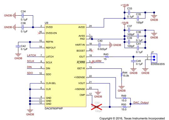
Figure 8. DAC8760 Schematic
