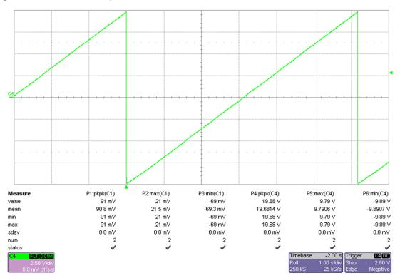
Figure 30. Monotonicity Check (Voltage Output)
