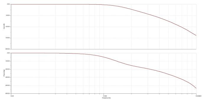
Figure 16. AC Transfer Function of S&H and Buffer Circuit
