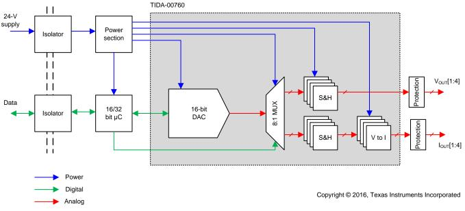
Figure 1. Generic S&H Multiplexed DAC PLC AO Module
