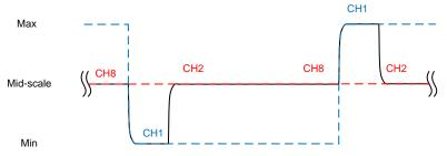
Figure 28. DAC Output in Full-Range Swinging Output Test
