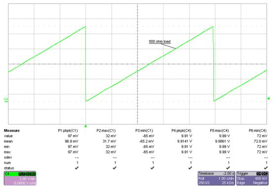
Figure 31. Monotonicity Check (Current Output)
