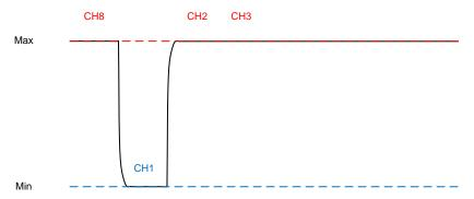
Figure 27. DAC Output in Output Test Where Channel 1 is Different Than Others
