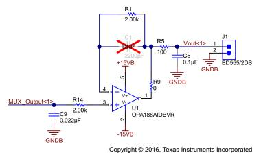
Figure 13. Buffer Circuit Schematic
