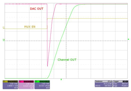
Figure 33. Positive Step Output Rise Time
