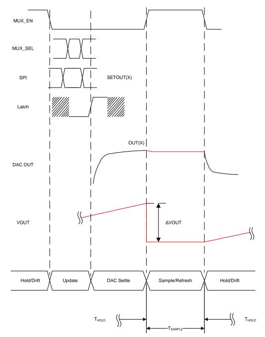
Figure 5. Detailed Channel Scan Cycle
