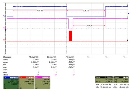
Figure 22. One Channel Update Cycle. C1: MUX\_EN, C4: LATCH, C3: SPI\_CLK
