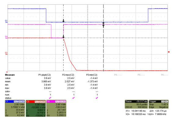
Figure 36. DAC Settling Time for Negative Step
