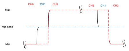
Figure 29. DAC Output in Crosstalk Output Test
