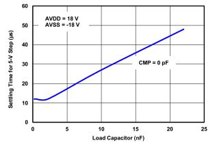
Figure 9. DAC V<sub>out</sub> Settling Time versus Load (CMP = 0 pF)
