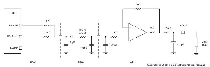
Figure 14. Signal Path Model (100-Ω Isolation Resistor)
