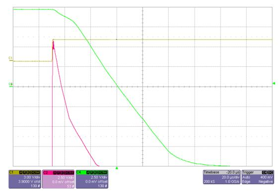
Figure 34. Negative Step Output Settling Time
