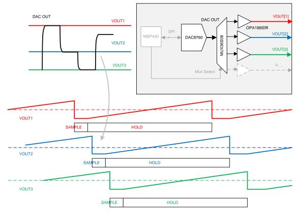
Figure 4. Concept of Multiplexed DAC S&H Outputs
