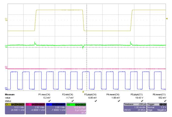
Figure 41. Waveform of Static Channel Affected by Nearby Toggling Channel
