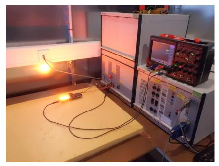
Figure 25. Setup for Transient Tests With LED Board and NSG 5500 Transient Generator
