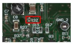
Figure 23. Resistor R32
