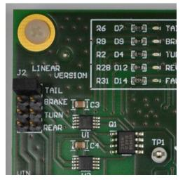
Figure 19. Jumper J2 for Setting the Type of Light
