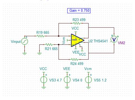
Figure 20. Simulation Circuit for THS4541 With Updated Gain of 0.750 V/V
