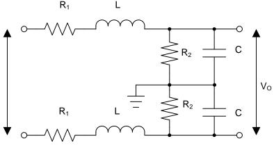
Figure 9. Differential Low-Pass RLC Filter
