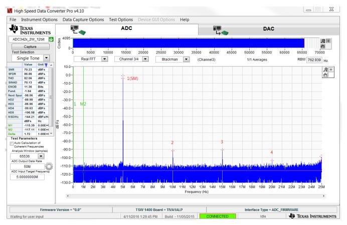
Figure 26. FFT Performance of Transformer Input
