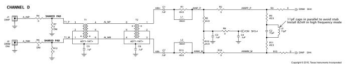
Figure 25. Transformer Coupled Input (Channel 4)
