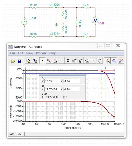
Figure 11. Simulation Circuit and Transfer Function for RLC Low-Pass Filter
