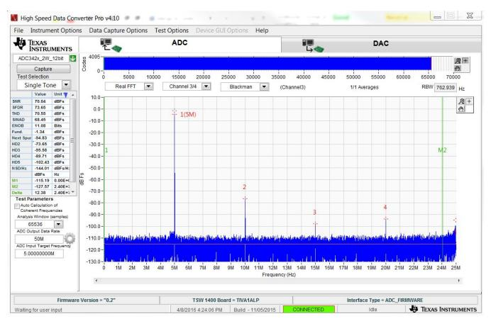
Figure 17. FFT Performance of Combined OPA656, THS4541, and RLC Low-Pass Filter
