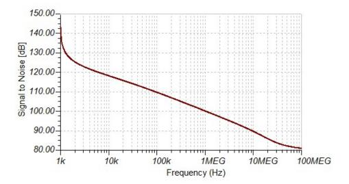
Figure 15. SNR for Complete OPA656 (JFET), Differential Amplifier (THS4541) With RLC Low-Pass Filter
