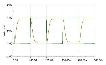
Figure 16. Simulation With ±1-V, 5-MHz Input Square Wave
