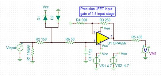
Figure 19. Simulation Circuit for OPA656 With Updated Gain of 1.5 V/V
