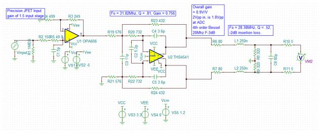
Figure 22. Channel 3 With Active, Second-Order, MFB Low-Pass Filter Stage
