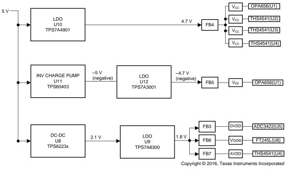
Figure 27. Power Supply Tree
