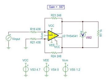
Figure 6. Simulation Circuit for Single-Ended to Differential Amplifier
