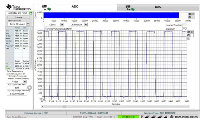
Figure 24. 1-MHz, ±1-V Square Wave Input
