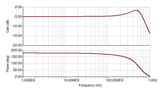
Figure 7. Transfer Function for Single-Ended to Differential Amplifier
