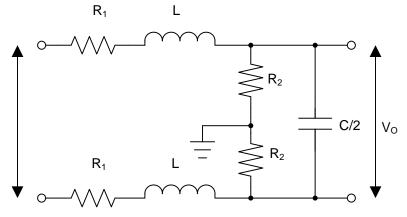
Figure 10. Simplified Differential Low-Pass Filter
