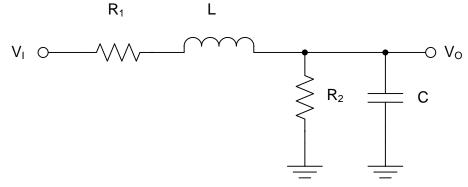
Figure 8. Single-Ended, Low-Pass RLC Filter
