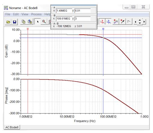
Figure 4. Transfer Function for OPA656 Stage
