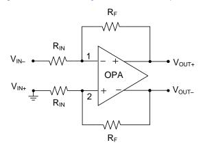
Figure 5. Single-Ended to Differential Amplifier
