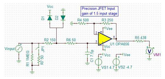
Figure 3. Simulation Circuit for OPA656
