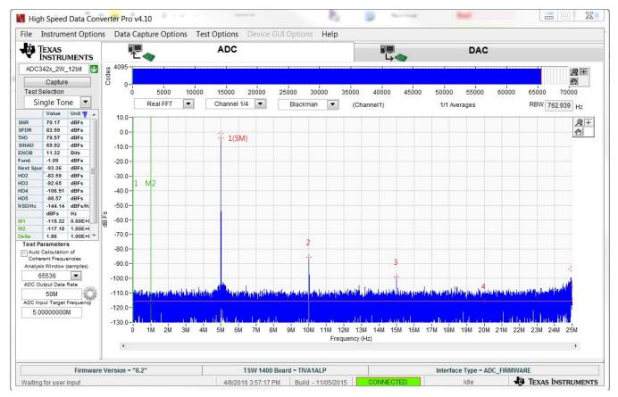
Figure 2. FFT Performance of THS4541 and ADC3422 Active Interface
