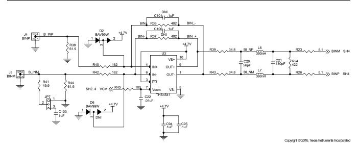
Figure 1. THS4541 Circuit Implementation With 20-MHz Cutoff Bessel LPF Driving ADC3422
