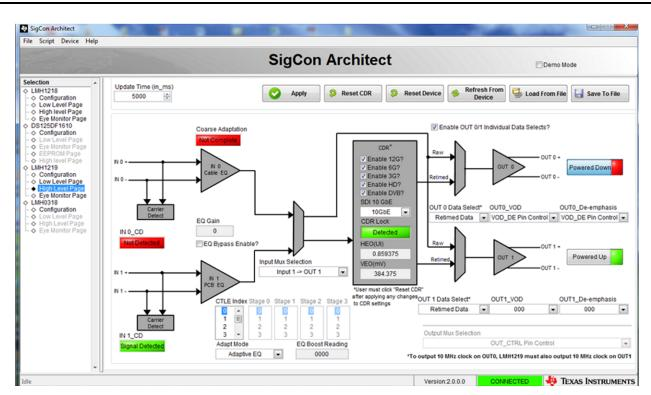
Figure 19. LMH1219 10-GbE GUI Setup
