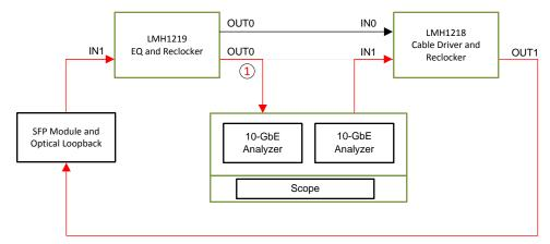
Figure 17. 10-GbE Optical Fiber Media Setup
