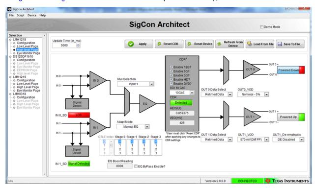
Figure 18. LMH1218 10-GbE GUI Setup
