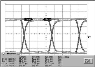
Figure 15. Output Eye Diagram PRBS10 2.97 Gbps at Point 5
