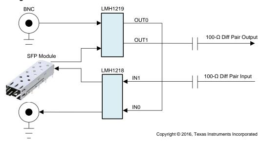
Figure 9. TIDA-00428 Block Diagram
