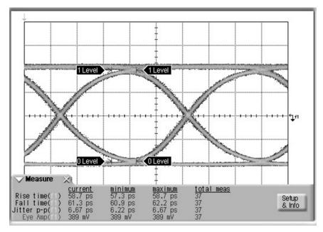
Figure 20. Output Eye Diagram PRBS10 10.3125 Gbps at Point 1
