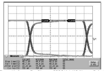
Figure 16. Output Eye Diagram PRBS10 1.485 Gbps at Point 5
