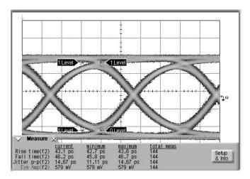
Figure 14. Output Eye Diagram PRBS10 11.88 Gbps at Point 5
