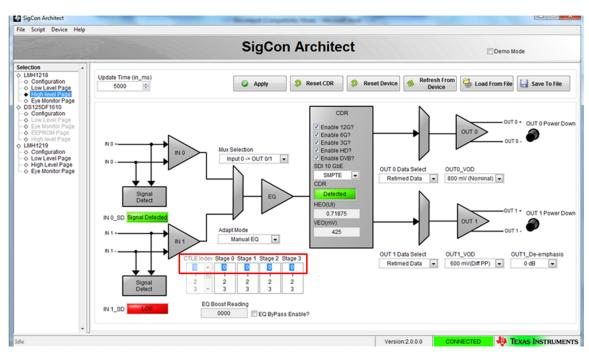
Figure 7. LMH1218 High Level GUI
