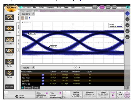
Figure 11. LMH1218 Eye Diagram at OUT0 Point 3
