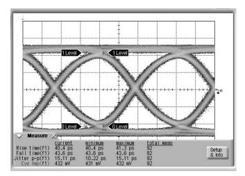
Figure 12. Output Eye Diagram PRBS10 11.88 Gbps at Point 6
