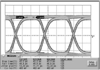
Figure 13. Output Eye Diagram PRBS10 5.94 Gbps at Point 6
