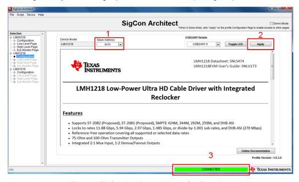
Figure 3. SigCon Architect LMH1218 Configuration
