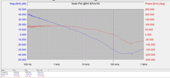
Vin=9V and Io=3A Fc=10.0KHz; Phase Margin=57.9°; Gain Margin=30.1dB
