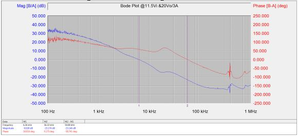
Vin=11.5V and Io=3A Fc=6.26KHz; Phase Margin=58.9°; Gain Margin=23.2dB
