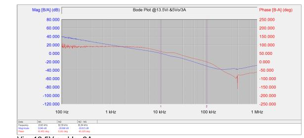
Vin=13.5V and Io=3A Fc=10.65KHz; Phase Margin=61.4°; Gain Margin=30dB
