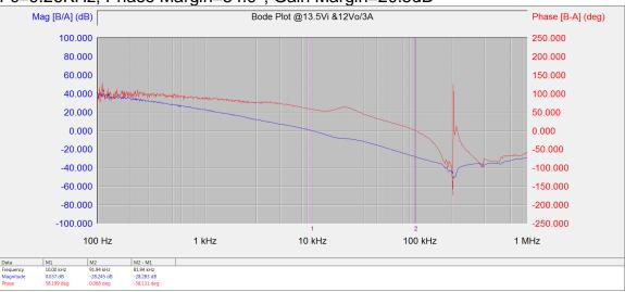
Vin=13.5V and Io=3A Fc=10.0KHz; Phase Margin=58.2°; Gain Margin=28.2dB
