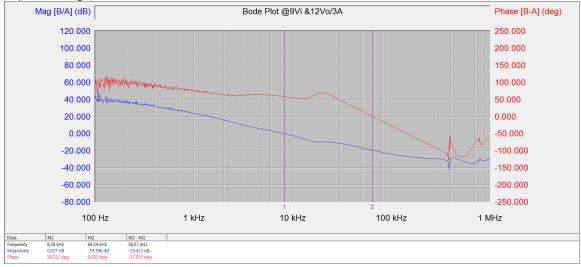
Vin=9V and Io=3A Fc=8.28KHz; Phase Margin=58.2°; Gain Margin=19.4dB
