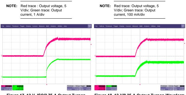
Figure 17. 12-V\_ISO/2.75-A Output Turnon Waveform at 400-V DC
