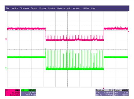
NOTE: Red trace: Output voltage, 10 V/div; Green trace: Output current, 2 A/div
