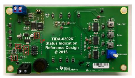
Figure 9. Audio Status Indication Test Setup
