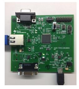
USB High Speed Reference Design for ARM<sup>®</sup> Cortex<sup>®</sup>-M4F Based High-Performance TM4C129x MCUs Copyright © 2016, Texas Instruments Incorporated
