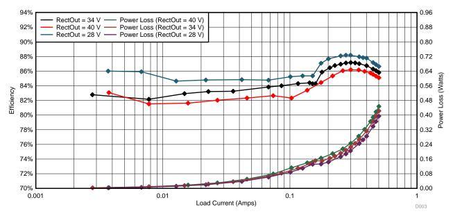
Figure 63. LM5166 Efficiency and Power Loss
