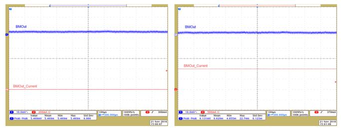
Figure 56. "BMOut" Ripple (0 A; Battery Source Only)
