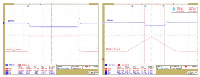
Figure 41. BM24072 Transient Response (250- to 750-mA; Battery and PWRin Source)
