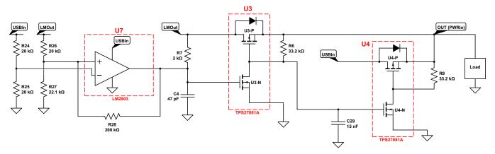
Figure 7. Power ORing Schematic
