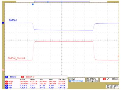
Figure 43. BM24702 Transient Response (250 to 750 mA; Battery Only)
