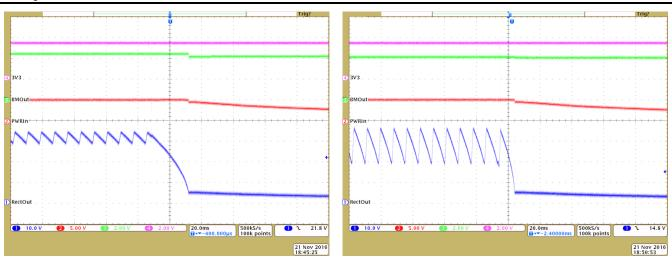
Figure 19. 24-V<sub>AC</sub> Shutdown (3V3 Load = 200 mA)
