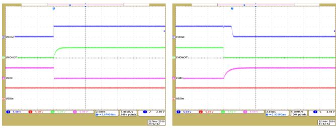
Figure 31. ORing Startup (LMOut Power Up; USB Source Present)
