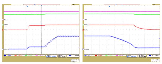
Figure 21. 20-V<sub>AC</sub> Startup
