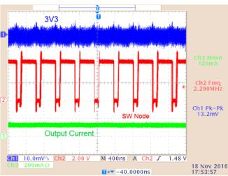
Figure 47. "3V3" Ripple Persist (120-mA Load; 24-V<sub>AC</sub> Source)
