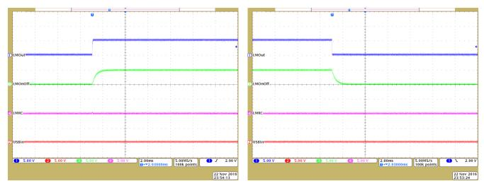
Figure 33. ORing Startup (LMOut Power Up; USB Source Absent)
