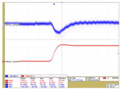
Figure 40. TLV62080 Transient Response Slew
