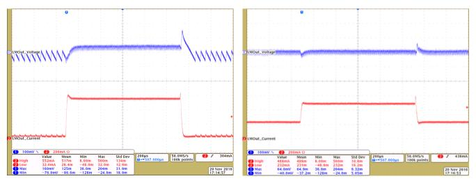
Figure 35. LM5166 Transient Response (0 to 480 mA)
