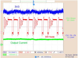
Figure 44. "3V3" Ripple (No Load; 24-V<sub>AC</sub> Source)
