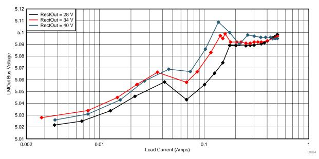
Figure 64. LM5166 Load Regulation
