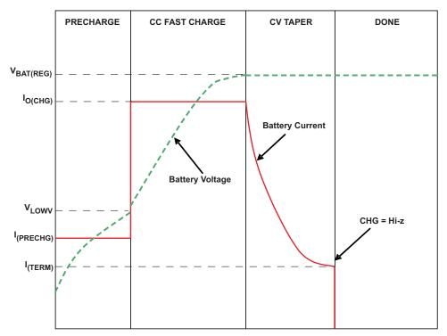
Figure 11. Typical Battery Charge Cycle
