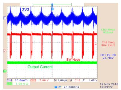
Figure 50. "3V3" Ripple Persist (1-A Load; Battery Powered Only)
