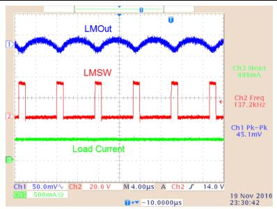
Figure 55. LMOut Ripple (490-mA Load)
