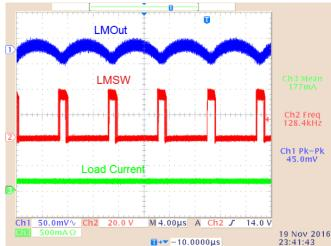
Figure 54. LMOut Ripple Persist (180-mA Load)
