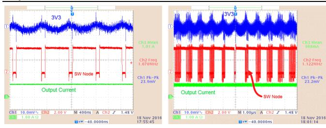
Figure 48. "3V3" Ripple (1-A Load; 24-V<sub>AC</sub> Source Plus Battery)
