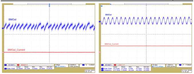
Figure 58. "BMOut" Ripple (1 mA; Battery and USB Sources)
