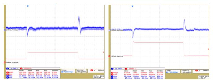
Figure 38. TLV61080 Transient Response (250 to 750 mA)
