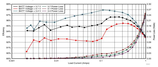
Figure 61. Battery to 3V3 Power Bus Efficiency and Power Loss
