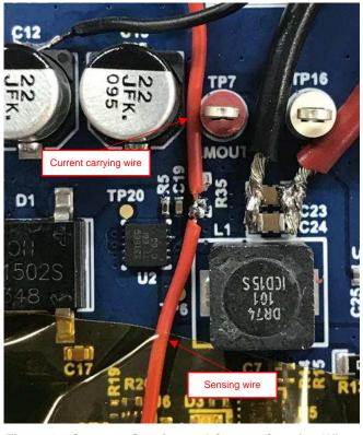
Figure 15. Current Probe and Electronic Load Test Setup
