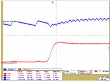
Figure 37. LM5166 Transient Response Slew
