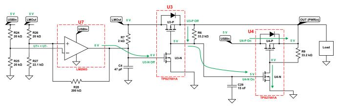
Figure 9. USB Supplied Power ORing
