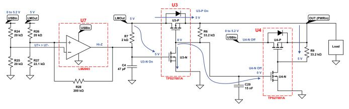
Figure 8. LM5166 Supplied Power ORing
