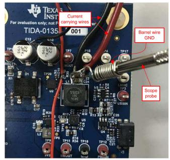
Figure 13. Soldered Output Wires Test Setup
