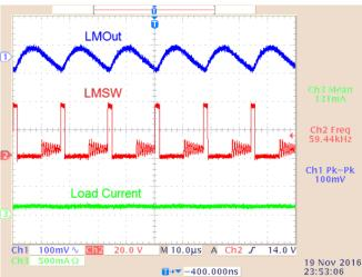
Figure 51. LMOut Ripple (No Load)
