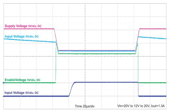
Figure 4. Overvoltage Protection
