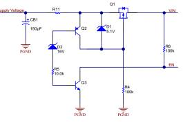
Figure 2. Overvoltage Protection Circuit Schematic
