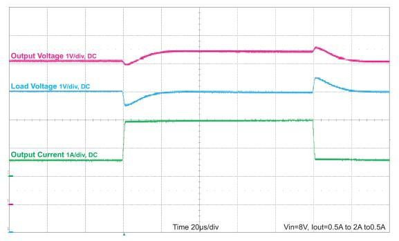
Figure 7. Load Transient
