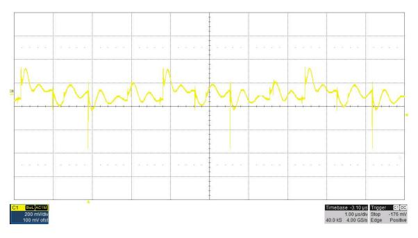
The 25V output ripple voltage (AC coupled) is shown in the figure below. The image was taken with the output loaded to 24A. The input voltage is set to 6V. (200mV/DIV, 1uS/DIV)
