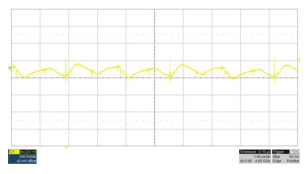
The input ripple voltage (AC coupled) is shown in the figure below. The image was taken with the output loaded to 24A. The input voltage is set to 6V. (100mV/DIV, 1uS/DIV)
