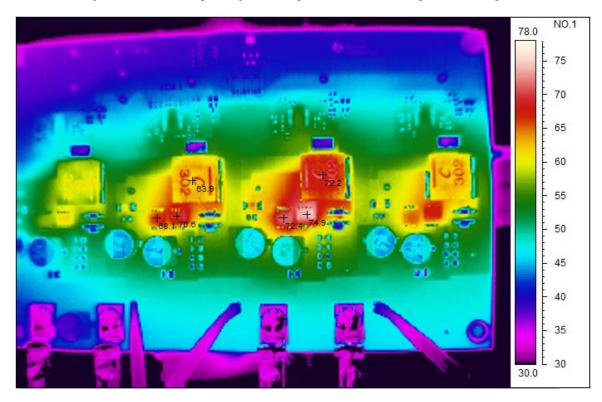
A thermal image is shown below operating at 12V input and 25V@24A output (room temp, no airflow).
