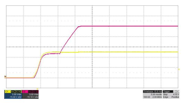
The photo below shows the output voltage startup waveform after the application of 12V in. The 25V output was loaded to 24A. (5V/DIV, 5mS/DIV)
