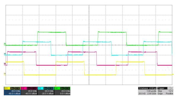
The photo below shows the FET switching voltages for an input voltage of 6V and a 24A load. (10V/DIV, 1uS/DIV)
