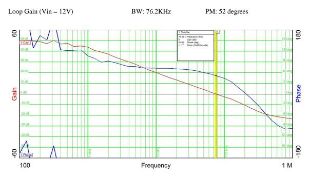
The plot below shows the LMR14030 5V USB loop gain for 12Vin and load of 2.1A. R33 opened.
