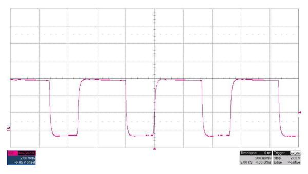
The photo below shows the **3.3VSW** switching voltage for an input voltage of 16V and a 2.5A load. (5V/DIV, 200nS/DIV)
