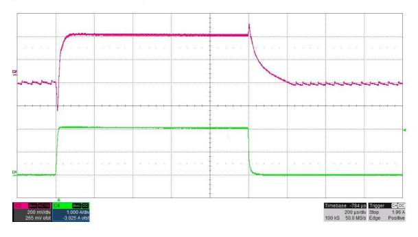
The **LMR14030 5V USB** load transient response (ac coupled) is shown for a load current step between 0A and 2.1A. Vin = 12V. The voltage is measured at R22 (0.2 Ohm resistor, after cable drop compensation). (200mV/DIV, 1A/DIV, 200uS/DIV)
