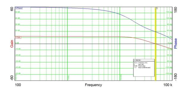
The plot below shows the TPS61175 LED Driver loop gain for 12Vin and a 3 white LED load (0.163A).
