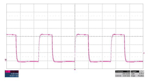
The photo below shows the **TPS57140 5V USB** switching voltage for an input voltage of 7V and a 1A load. (2V/DIV, 200nS/DIV)
