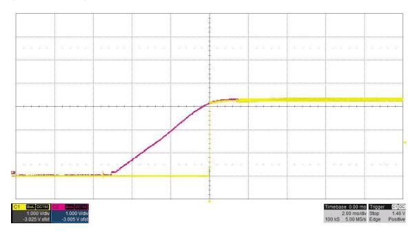
The photo below shows the **12V ANT** startup waveforms after 12V is applied. 12Vin (Red), 12V ANT (Yellow), 50mA loads on output, 12V ANT ENABLE connected to Vin. (2V/DIV, 200uS/DIV)
