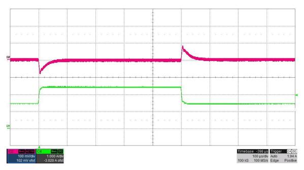
The **3.3VSW** load transient response (ac coupled) is shown for a load current step between 0.5A and 2.5A. Vin = 12V.
