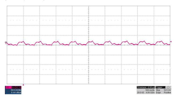
The **LMR14030 5V USB** output ripple voltage (AC coupled) is shown in the figure below. The voltage is measured across C28 with the output loaded to 2.1A. The input voltage is set to 16V. (50mV/DIV, 500nS/DIV)
