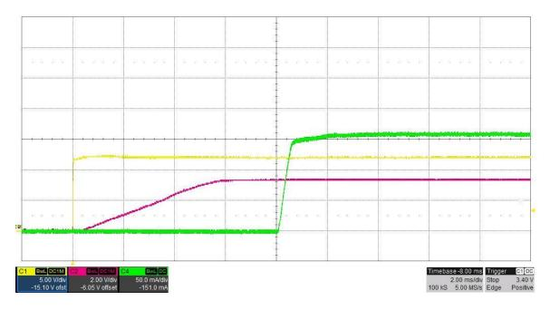
The photo below shows the **TPS61175 LED** current startup waveform after the EN signal (Red) is applied. 3.3VSW (Yellow), TPS61175 Enable (Red), TPS61175 LED current (Green), 3 White LED, 3.3VSW@1A (2V/DIV, 50mA/DIV, 2mS/DIV)
