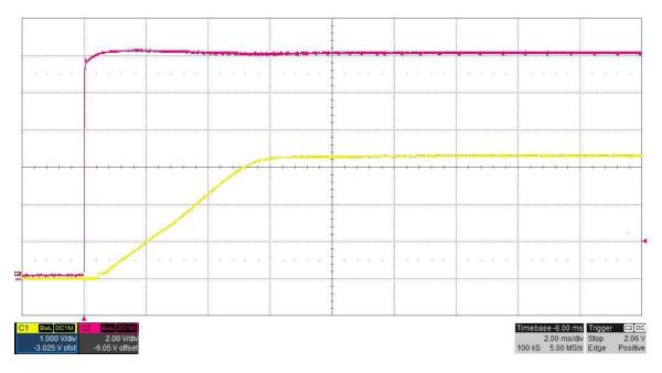
The photo below shows the **3.3VSW** output voltage startup waveform after 12V is applied. VIN (Red), 3.3VSW (Yellow), 3.3V output is loaded to 2.5A. (VIN is 2V/DIV, 3.3V is 1V/DIV, 2mS/DIV)
