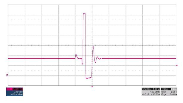
The photo below shows the **LMR14030 5V USB** switching voltage for an input voltage of 7V and a 2.1A load. (2V/DIV, 200nS/DIV)
