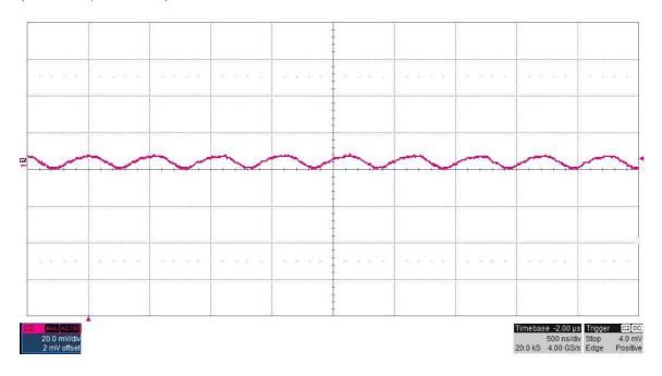
The **TPS57140 5V USB** output ripple voltage (AC coupled) is shown in the figure below. The voltage is measured across C45 with the output loaded to 1A. The input voltage is set to 16V. (20mV/DIV, 500nS/DIV)
