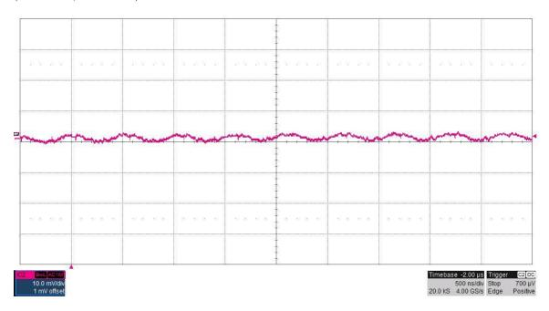
The **3.3VSW** output ripple voltage (AC coupled) is shown in the figure below. The voltage is measured across C16 with the output loaded to 2.5A. The input voltage is set to 16V. (10mV/DIV, 500nS/DIV)
