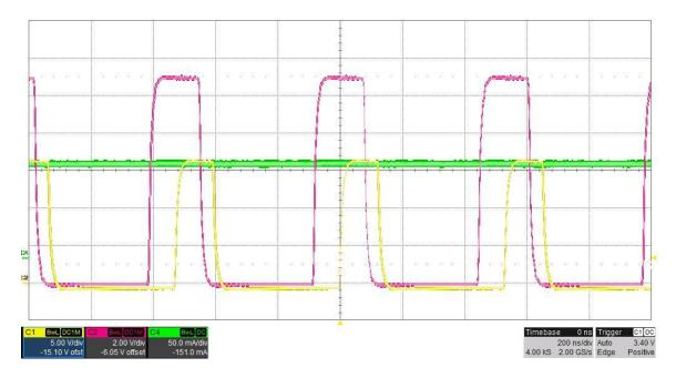
The photo below shows the **TPS61175 LED driver** switching voltage for an input voltage of 12V with open LEDs (fault condition). 3.3VSW@1A
