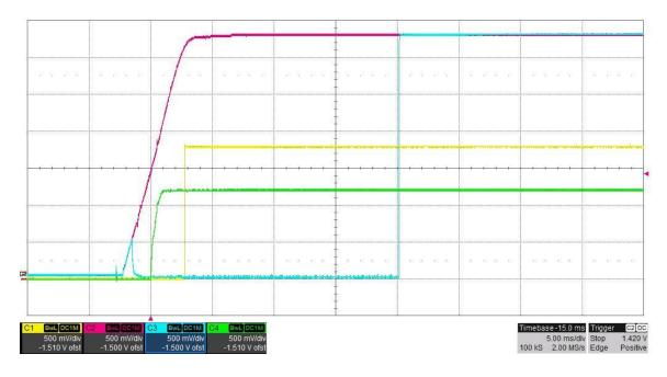
The photo below shows the **5V STBY**, **3.3V STBY**, **and 3.3V MIC** startup waveforms after 12V is applied. 12Vin (Red), 5V STBY (Blue), 3.3V STBY (Green), 3.3V MIC (Yellow), 0A loads on all outputs. (2V/DIV, 100uS/DIV)
