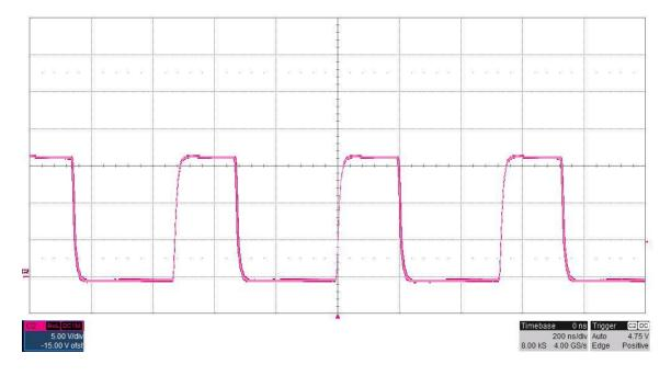
The photo below shows the **TPS61175 LED driver** switching voltage for an input voltage of 6V and driving 3 white LEDs. 3.3VSW@1A
