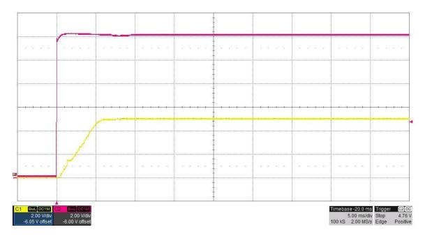
The photo below shows the **LMR14030 5V USB** output voltage startup waveform after 12V is applied. VIN (Red), LMR14030 5V USB (Yellow), 5V output is loaded to 2.1A. (2V/DIV, 5mS/DIV)
