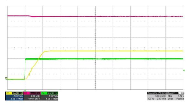
The photo below shows the **TPS57140 5V USB** output voltage startup waveform after 12V is applied. VIN (Red), TPS57140 5V USB (Blue), 5V output is loaded to 0A. (2V/DIV, 5mS/DIV)
