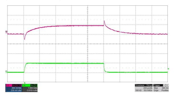
The **TPS57140 5V USB** load transient response (ac coupled) is shown for a load current step between 0A and 1A. Vin = 12V. The voltage is measured at R35 (0.2 Ohm resistor, after cable drop compensation). (200mV/DIV, 1A/DIV, 200uS/DIV)
