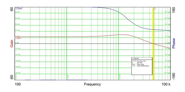
The plot below shows the **TPS57140 5V USB** loop gain for 12Vin and load of 1A. R48 opened.
