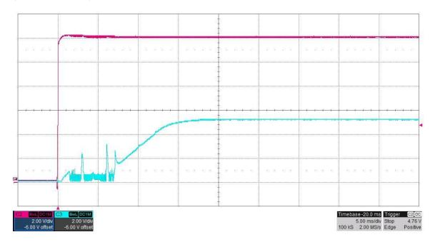
The photo below shows the **TPS57140 5V USB** output voltage after the EN signal (Green) is applied. VIN (Red), TPS57140 5V USB (Blue), 5V output is loaded to 1A. Vin =12V (2V/DIV, 5mS/DIV)
