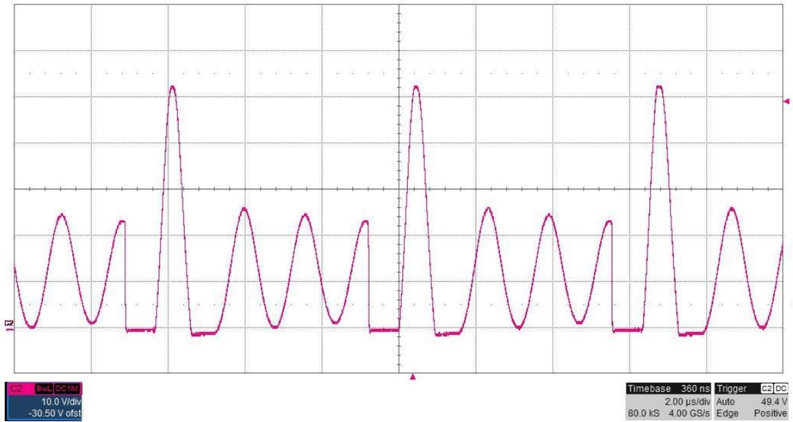
The photo below shows the FET switching voltage (TP2) for an input voltage of 40V and a 0A load. (10V/DIV, 10uS/DIV)
