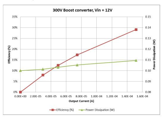
The converter efficiency is shown below for Vin = 12V and Vout = 150V.
