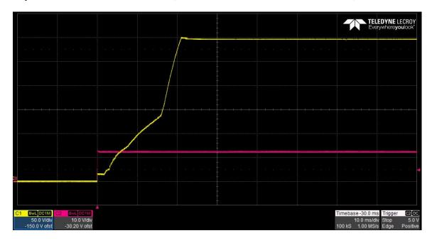
The photo below shows the output voltage startup waveform after the application of 12V in. The 150V output was loaded to 0A. Vcontrol = 3V, (Vin is 10V/DIV, Vout is 50V/DIV, 10mS/DIV)
