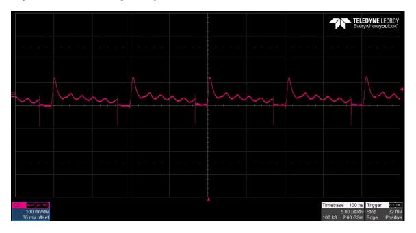
The 150V output ripple voltage (AC coupled) is shown in the figure below. The image was taken with the output loaded to 25uA. The input voltage is set to 9V. (100mV/DIV, 5uS/DIV)
