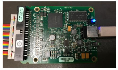
Figure 25. NI USB-8452 Interface Board
