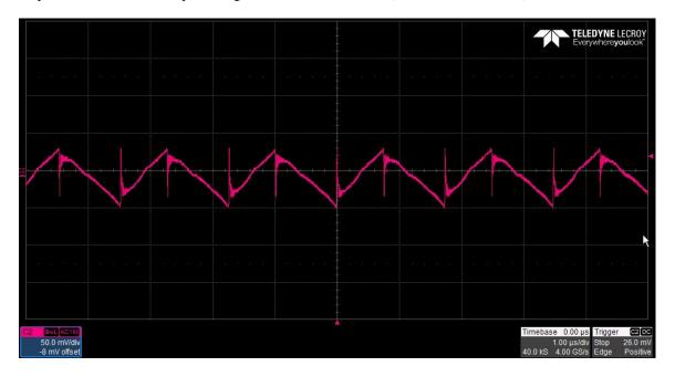
The 7V output ripple voltage (AC coupled) is shown in the figure below. The image was taken with the output loaded to 3A. The input voltage is set to 16V. (50mV/DIV, 1uS/DIV)
