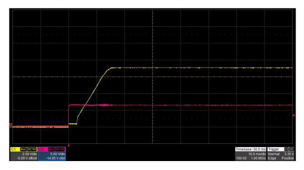
The photo below shows the output voltage startup waveform after the application of 6.5V in. The 7V output was loaded to 3A. (Vin is 5V/DIV, Vout is 2V/DIV, 10mS/DIV)
