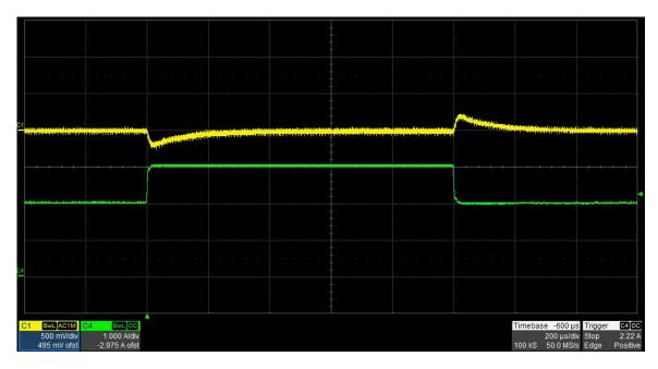
The photo below shows the 7V output voltage (ac coupled) when the load current is stepped between 1A and 3A. Vin = 12V. (500mV/DIV, 1A/DIV, 200uS/DIV)
