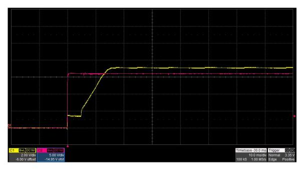
The photo below shows the output voltage startup waveform after the application of 16V in. The 7V output was loaded to 3A. (Vin is 5V/DIV, Vout is 2V/DIV, 10mS/DIV)
