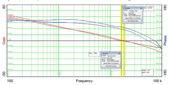
The plot below shows the loop gain with the input voltage set to 6.5V and 16V with the output set to 0.75A.
