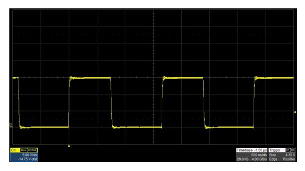
The photo below shows the FET switching voltage for an input voltage of 16V and a 3A load. (5V/DIV, 500nS/DIV)
