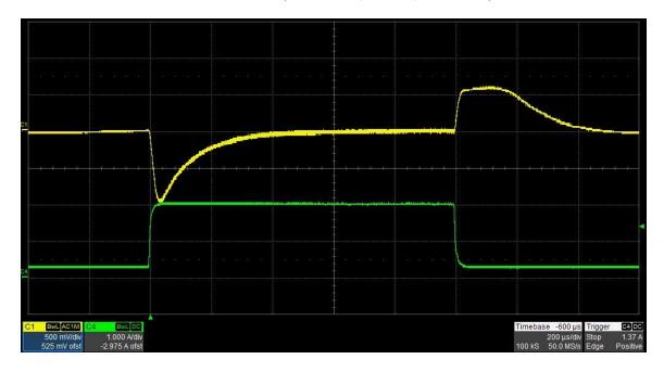
The photo below shows the 10V output voltage (ac coupled) when the load current is stepped between 0A and 2A. Vin = 12V. (1V/DIV, 1A/DIV, 200uS/DIV)
