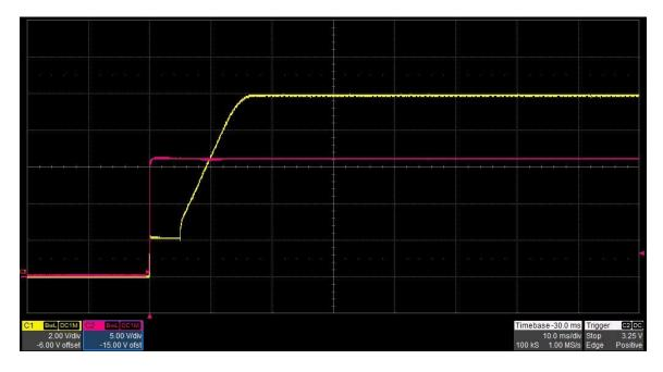
The photo below shows the output voltage startup waveform after the application of 16V in. The 10V output was loaded to 2A. (Vin is 5V/DIV, Vout is 2V/DIV, 10mS/DIV)
