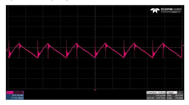
The 10V output ripple voltage (AC coupled) is shown in the figure below. The image was taken with the output loaded to 2A. The input voltage is set to 16V. (50mV/DIV, 1uS/DIV)
