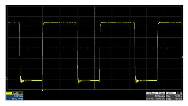
The photo below shows the FET switching voltage for an input voltage of 16V and a 0.45A load. The converter is operating in DCM. (5V/DIV, 500nS/DIV)
