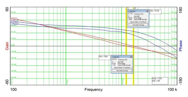
The plot below shows the loop gain with the input voltage set to 6.5V and 16V with the output set to 0.5A.
