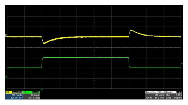
The photo below shows the 10V output voltage (ac coupled) when the load current is stepped between 0.5A and 2A. Vin = 12V. (500mV/DIV, 1A/DIV, 200uS/DIV)
