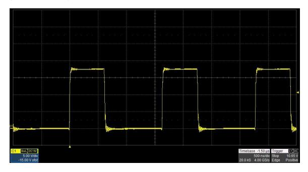
The photo below shows the FET switching voltage for an input voltage of 12V and a 2A load. (5V/DIV, 500nS/DIV)
