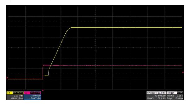
The photo below shows the output voltage startup waveform after the application of 6.5V in. The 10V output was loaded to 2A. (Vin is 5V/DIV, Vout is 2V/DIV, 10mS/DIV)
