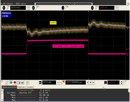
12Vin, 1.0Vout, 45A to 60A Load Step, -15mV (-1.5%), +15mV (+1.5%)
