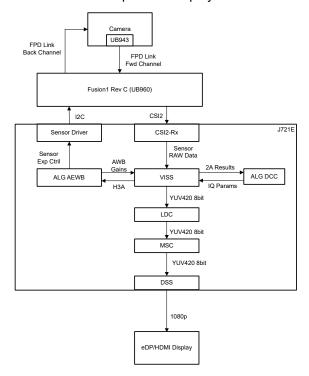
Figure 3-2. Test Setup
