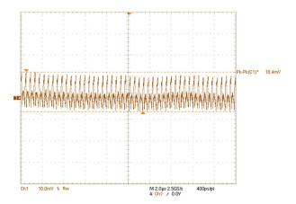
Figure 3-6. Output Voltage Ripple - 3.3 V
