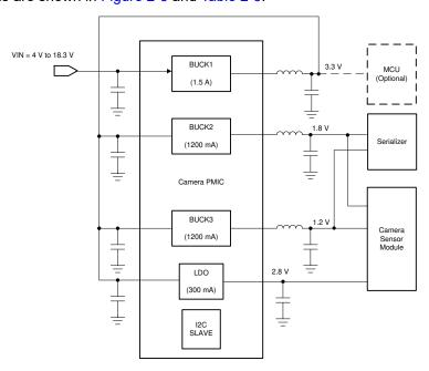
Figure 2-5. TPS650330-Q1 Typical Application Circuit
