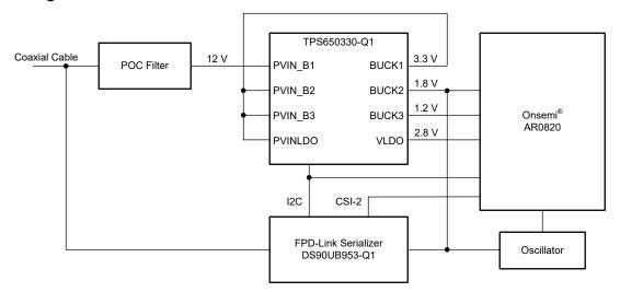
Figure 2-1. Camera Block Diagram
