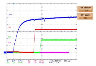
(Channel 1): 12-V supply; (Channel 2): 2.8-V supply; (Channel 3): 1.8-V supply; (Channel 4): PDB
