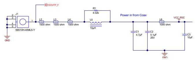
Figure 1-1. FPD-Link III Signal Path
