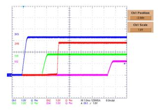
(Channel 1): 3.3-V supply; (Channel 2): 2.8-V supply; (Channel 3): 1.8-V supply; (Channel 4): 1.2-V supply
