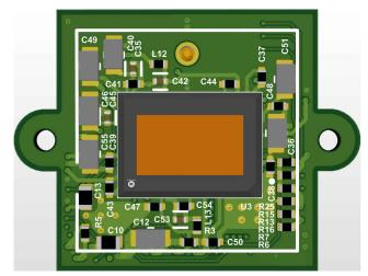
Figure 2-2. 3-D PCB Top Layer
