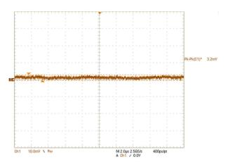
Figure 3-7. Output Voltage Ripple - 2.8 V
