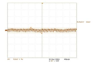
Figure 3-9. Output Voltage Ripple - 1.2 V
