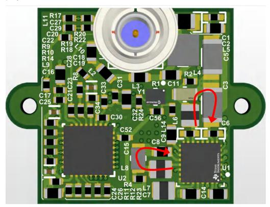
Figure 4-1. PMIC PCB Layout
