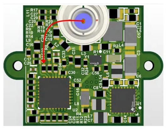
Figure 4-2. High-Speed Trace Routing
