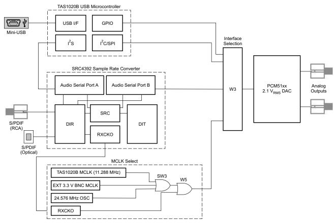
Figure 2. PCM5122/42EVM-U Block Diagram
