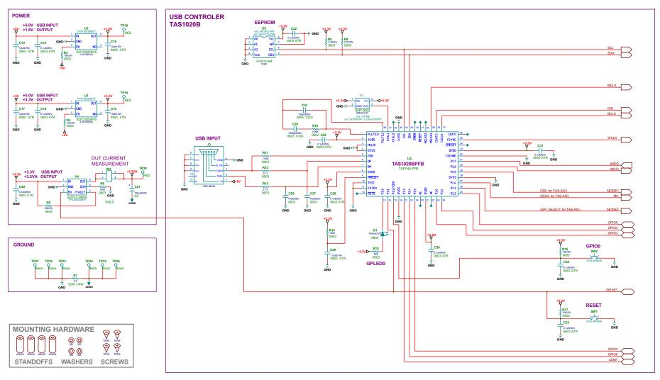
Figure 9. PCM514xEVM-U Power and USB Controller
