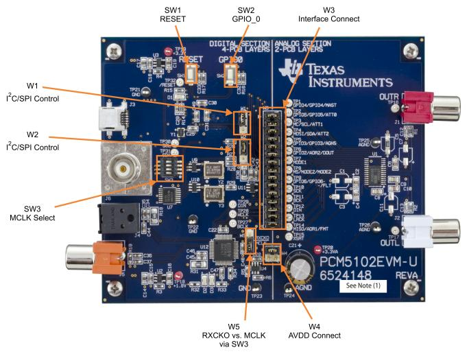
(1) The silkscreen label shown on the board may be different to indicate a specific device. Otherwise, the EVM is identical to the one shown here.
