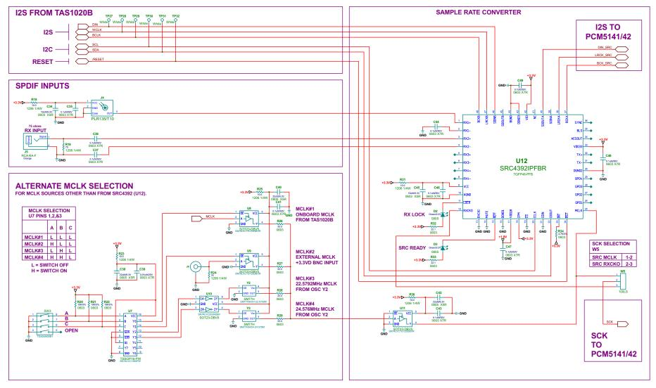
Figure 10. PCM514xEVM-U Digital I/O and Source
