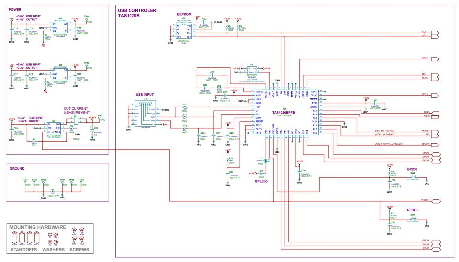
Figure 6. PCM512xEVM-U Power and USB Controller
