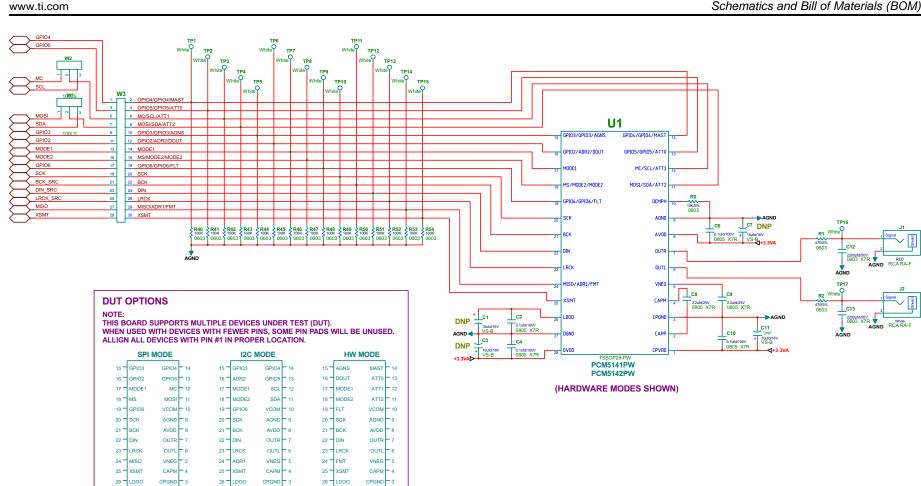
Figure 8. PCM514xEVM-U Schematic
