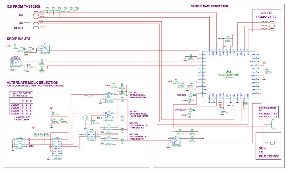
Figure 7. PCM512xEVM-U Digital I/O and Source
