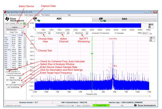
Figure 3-5. High Speed Data Converter Pro (HSDC) GUI
