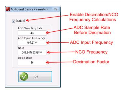
Figure 3-6. Additional Device Parameters Tab
