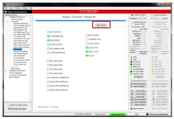
Figure 7. TLK10022/81 EVM GUI High Level Device Status Windows
