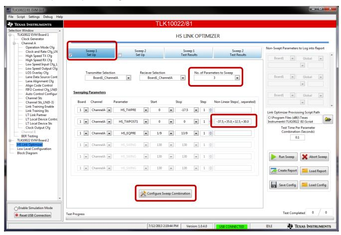
Figure 12. TLK10022/81 EVM GUI High Speed Link Optimizer Setup
