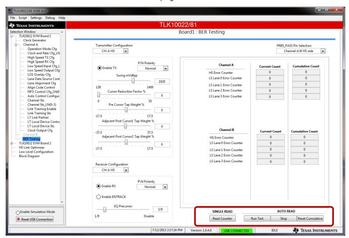
Figure 11. TLK10022/81 EVM GUI High Level BER Testing
