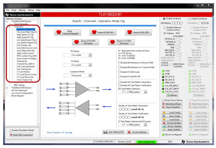
Figure 2. TLK10022/81 EVM GUI Hierarchical Selection Window Tree
