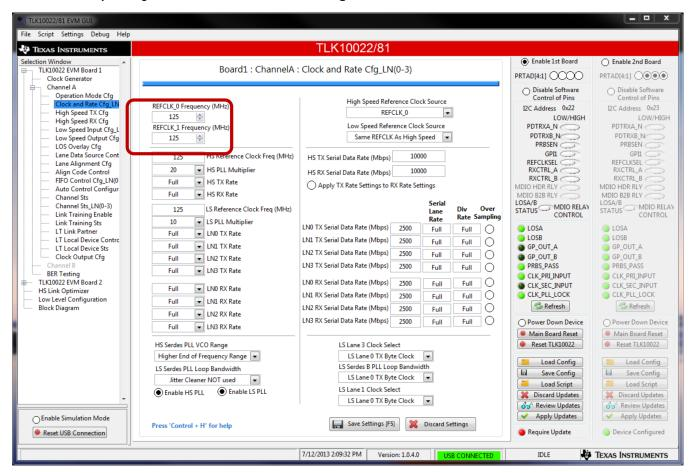
Figure 6. TLK10022/81 EVM GUI High Level Device Clock and Rate Configuration
