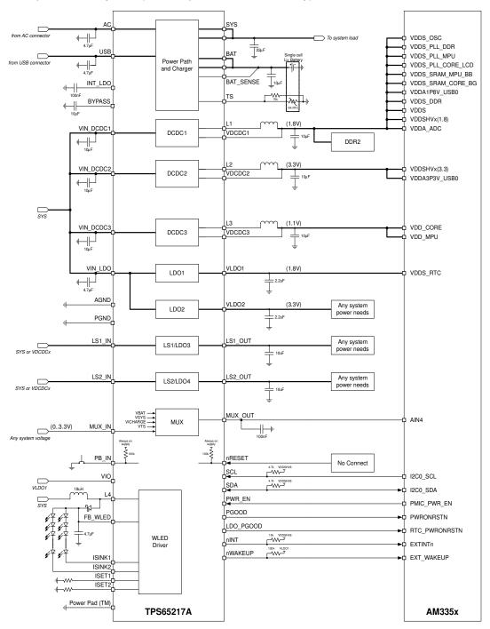
Figure 1. Connection Diagram for TPS65217A and AM335x
