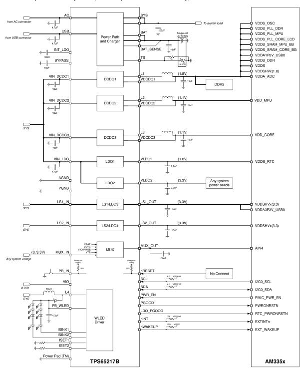
Figure 3. Connection Diagram for TPS65217B and AM335x
