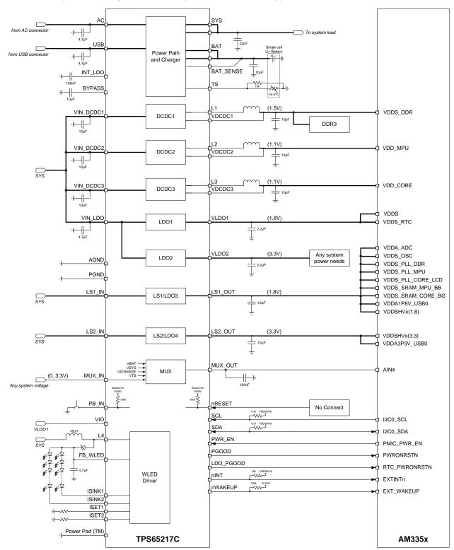
Figure 5. Connection Diagram for TPS65217C and AM335x
