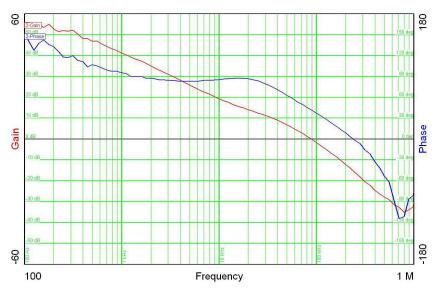
Figure 5. TPS54388EVM Loop-Response Measurement
