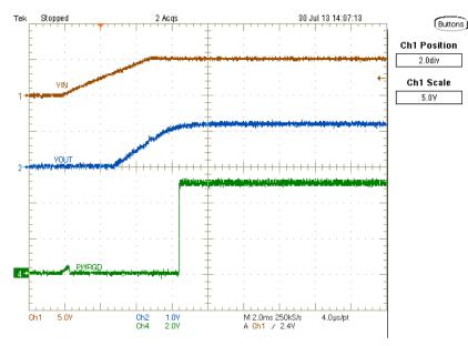
Figure 7. TPS54388EVM Startup Relative to V<sub>IN</sub>
