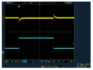
Figure 4. TPS54388EVM Load Transient
