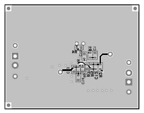
Figure 12. TPS54388EVM Bottom-Side Assembly
