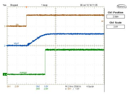
Figure 8. TPS54388EVM Startup Relative to Enable
