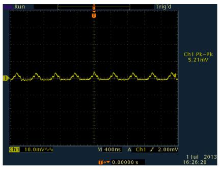
Figure 6. TPS54388EVM Output Ripple
