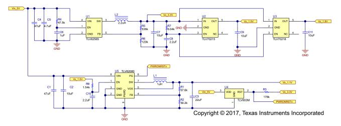
Figure 3. Powering and Sequencing Circuit for AM437x Requirements
