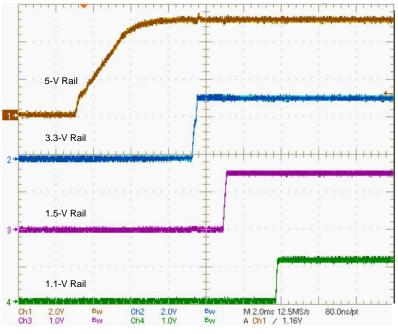
Figure 4. Power-On Sequence with Converter Rails
