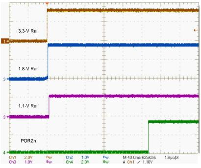
Figure 6. Power-On Sequence with PORZn Signal
