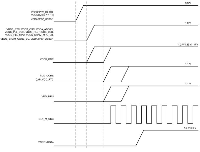
Figure 2. Power-On Sequence for AM437x
