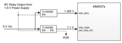
Figure 12. Block Diagram of 1-GHz Mode Support
