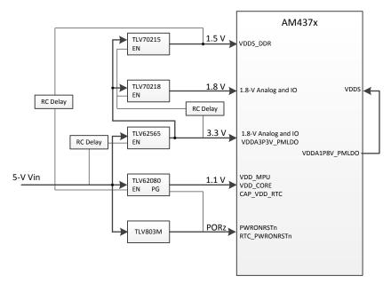
Figure 1. Functional Block Diagram Powering AM437x
