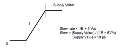
Figure 11. Power Supply Slew Rate Requirement
