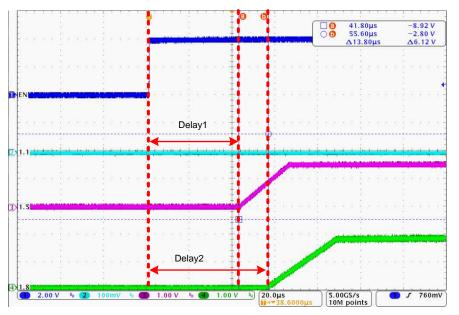
Figure 10. Potentially Different Delays with Sharp EN Signal
