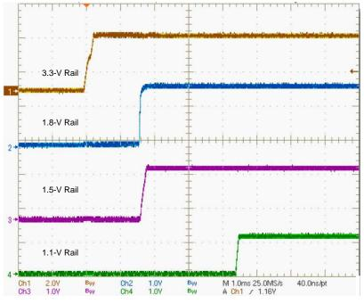
Figure 5. Power-On Sequence for AM437x
