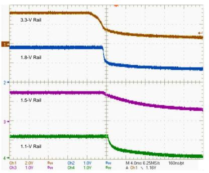
Figure 8. Power-Off Sequence with All Power Supply Rails
