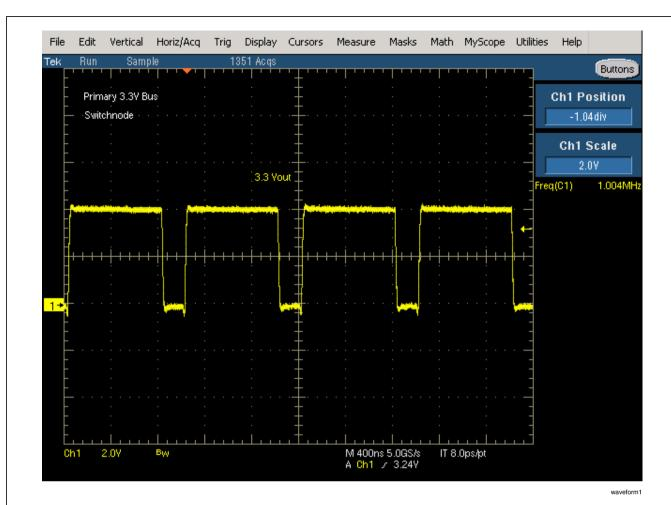
FIGURE 7. Primary 3.3V Bus - Switchnode Voltage
