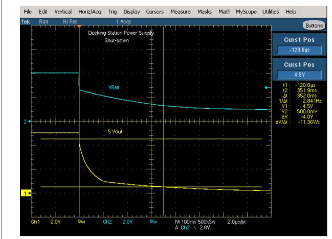
FIGURE 15. Docking Station Power Supply - Shut-down Waveform
