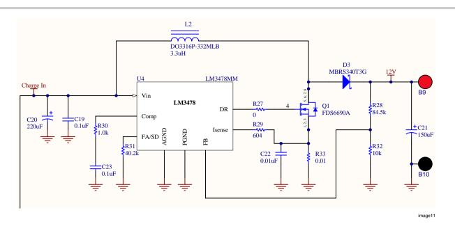
FIGURE 21. Video Interface (LCD) Controller Power Supply Schematic
