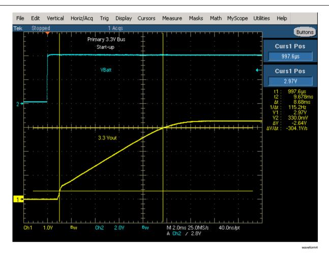
FIGURE 12. Primary 3.3V Bus - Start-up Waveform
