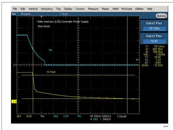
FIGURE 17. Video Interface Controller Power Supply - Shut-down Waveform
