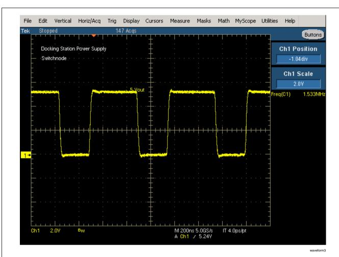
FIGURE 9. Docking Station Power Supply - Switchnode Voltage
