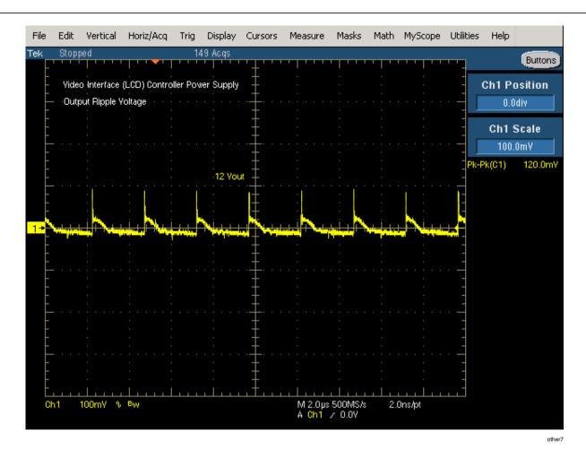
FIGURE 10. Video Interface Controller Power Supply - Output Ripple Voltage
