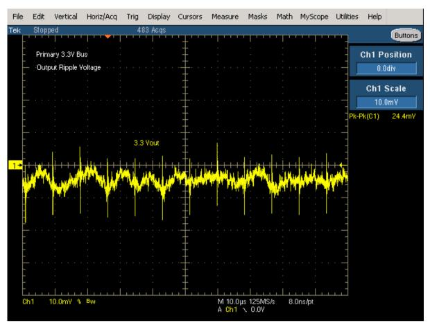
FIGURE 6. Primary 3.3V Bus - Output Ripple Voltage
