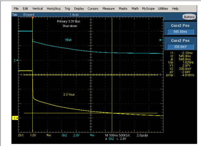
FIGURE 13. Primary 3.3V Bus - Shut-down Waveform
