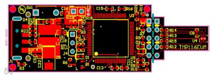
Figure 21. Top Assembly Layer
