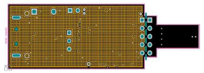
Figure 24. Ground Layer Routing
