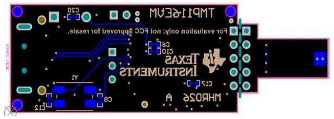
Figure 26. Bottom Assembly Layer
