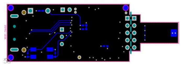
Figure 25. Bottom Layer Routing
