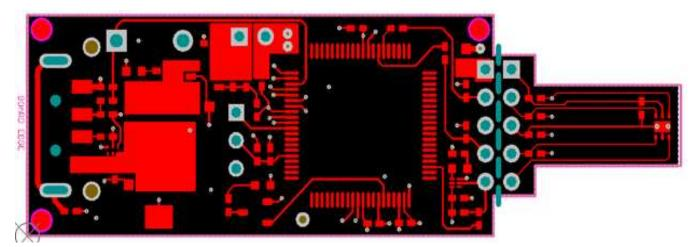
Figure 22. Top Layer Routing
