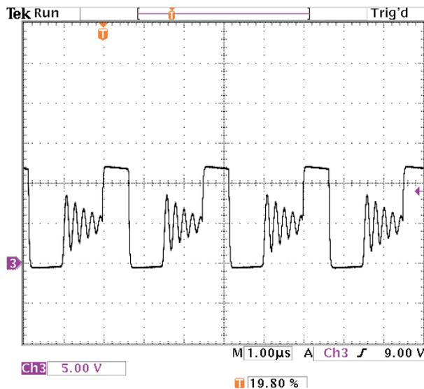
Scope Measurements: Vin = 12 V, Vout = 5 V, Iout = 300 mA
