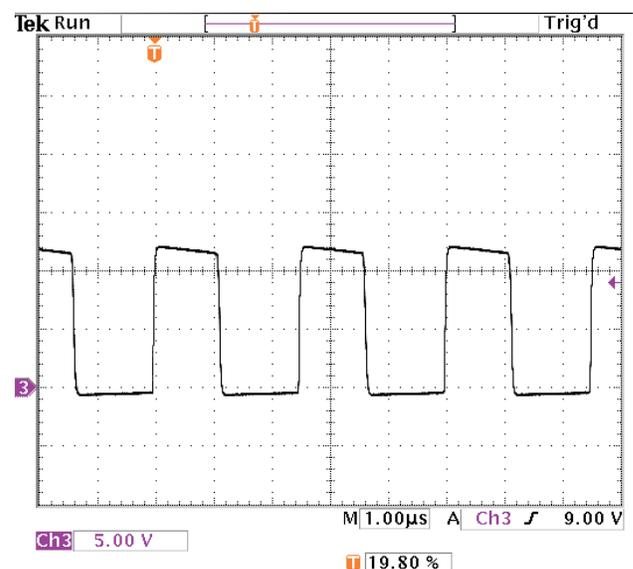
Scope Measurements: Vin = 12 V, Vout = 5 V, Iout = 1.0 A
