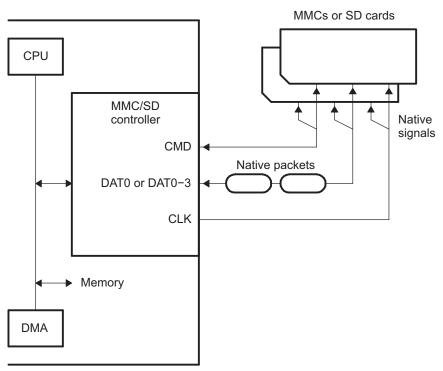
Figure 10-2. MMC/SD Controller Interface Diagram
