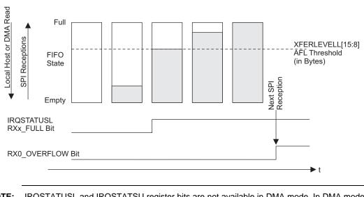
Figure 9-20. Buffer Almost Full Level (AFL)
