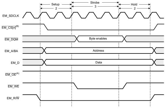
A. During the entirety of an asychronous write operation, the EM\_OE pin is driven high.
