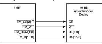
Figure 4-9. Common Asynchronous Interface
