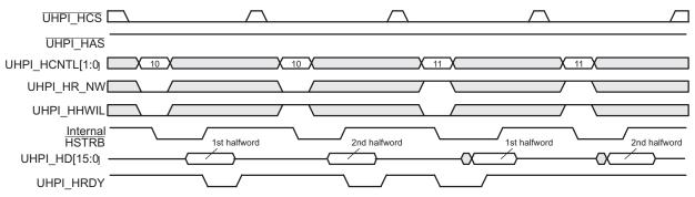
Figure 16-10 includes an autoincrement UHPID read cycle. The host writes the memory address while asserting UHPI\_HCNTL[1:0] = 10b and reads the data while asserting UHPI\_HCNTL[1:0] = 01b. During the first UHPID read cycle, UHPI\_HRDY goes low for only the first halfword access, and subsequent UHPID read cycles do not cause UHPI\_HRDY to go low.
