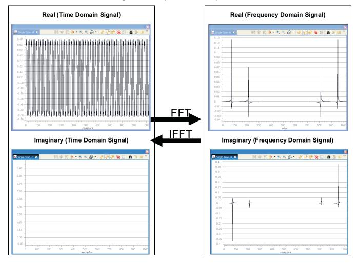
Figure 2-3. Graphical FFT Computation
