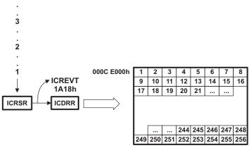
Figure 3-9. Servicing Incoming I2C Data Example DMA Configuration
