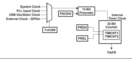
**NOTE:** The timer architecture also includes logic, not shown, to synchronize parts of the timer circuit running on the internal timer clock with an asynchronous input clock source.
