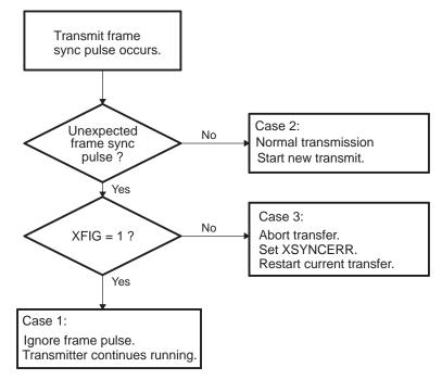
Figure 8-30. Decision Tree Response to Transmit Frame Synchronization Pulse
