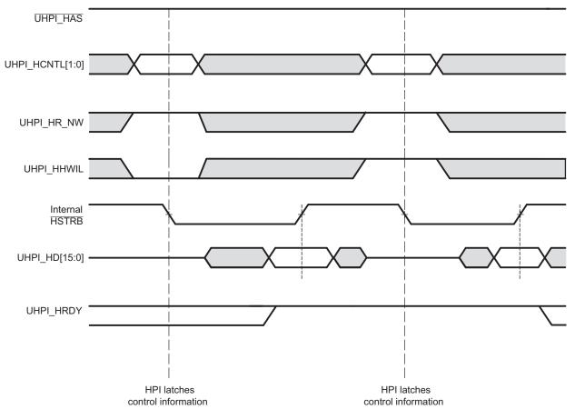
Figure 16-4. Host Read without UHPI\_HAS (Dual Half-Word Cycle)
