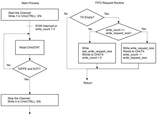
Figure 9-36. FIFO Mode Transmit-Only (Master)
