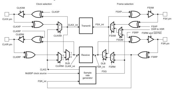
Figure 8-2. Clock and Frame Generation
