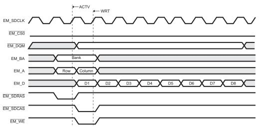
Figure 4-6. Timing Waveform for Basic SDRAM Write Operation
