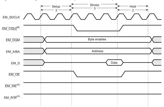
Figure 4-12. Timing Waveform of an Asynchronous Read Cycle in Select Strobe Mode
