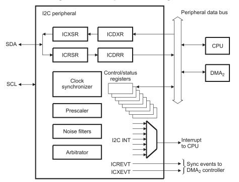
Figure 6-1. I2C Peripheral Block Diagram
