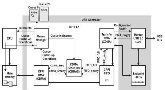
Figure 17-21. Receive USB Data Flow Example (Initialization)
