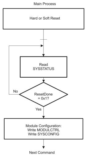
**NOTE:** Before the SYSSTATUSL[0] RESETDONE bit is set, the CLK and CLKSPIREF clocks must be provided to the module.
