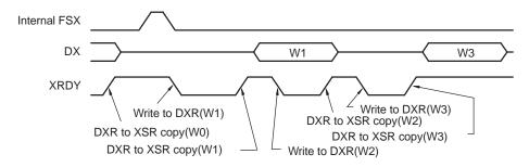
(d) XMCM = 3h, RPABLK = 0, XPABLK = x, RCEREA = 0008h, XCEREA = 000Ah: Receive channels: 1 and 3 enabled; transmit channels: 1 and 3 enabled, but only 3 unmasked
