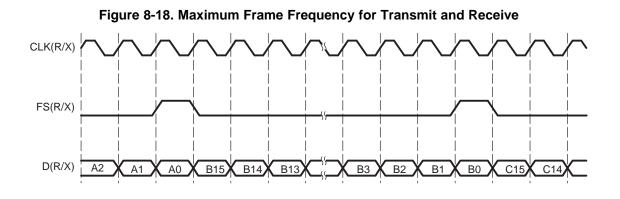
**NOTE:** For (R/X)DATDLY = 0, the first bit of data transmitted is asynchronous to CLKX, as shown in Figure 8-13.
