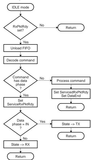
Figure 17-8. IDLE Mode Flow Chart
