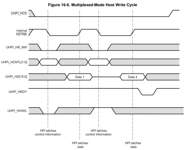
NOTE: Depending on the type of write operation (UHPID without autoincrementing, UHPIA, UHPIC, or UHPID with autoincrementing) and the state of the FIFO, transitions on UHPI\_HRDY may or may not occur. For more information, see Section 16.2.5.10.
