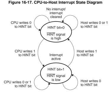
If the CPU writes 1 to the HINT bit of UHPIC, the UHPI drives the UHPI\_HINT signal low, indicating an interrupt condition to the host. Before the CPU can use the HINT bit generate a subsequent interrupt to host, the host must acknowledge the current interrupt by writing 1 to the HINT bit. When the host does this, the UHPI clears the HINT bit (HINT = 0), and this drives the UHPI\_HINT signal high. The CPU should read UHPIC and make sure HINT = 0 before generating subsequent interrupts.
