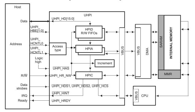
Figure 16-1. UHPI Block Diagram
