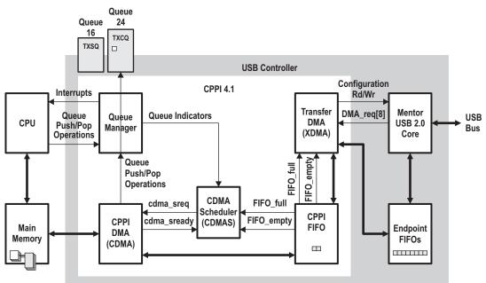
Step 4 (Return packet to completion queue and interrupt CPU for Tx):
