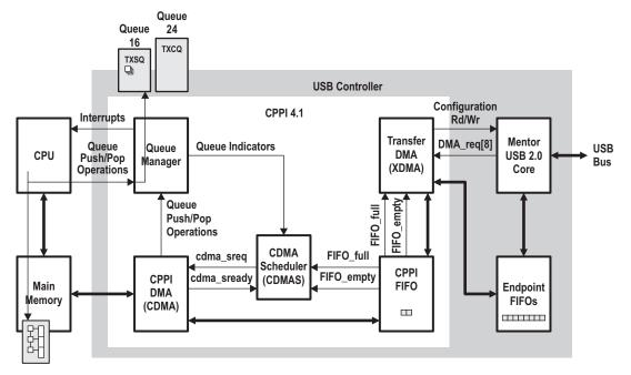
Figure 17-18. Transmit USB Data Flow Example (Initialization)
