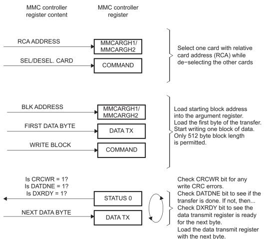
Figure 10-13. MMC/SD Mode Single-Block Write Operation
