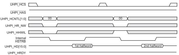
Figure 16-12 includes a UHPID write cycle without autoincrementing. The host writes the memory address while UHPI\_HCNTL[1:0] = 10b and writes the data while UHPI\_HCNTL[1:0] = 11b. During the UHPID write cycle, UHPI\_HRDY goes low only for the second halfword access.
