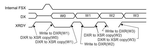
(b) XMCM = 1h, XPABLK = 0, XCEREA = 000Ah: Only channels 1 and 3 enabled and unmasked
