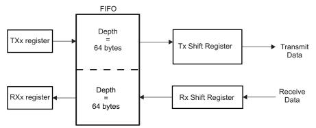
Two levels, XFERLEVELU[15:8] AFL and XFERLEVELL[7:0] AEL, rule the buffer management. The granularity of these levels is one byte, then it is not aligned with SPI word length. It is the responsibility of the driver to set these values as a multiple of SPI word length defined in WL. Table 9-5 shows the number of byte written in the FIFO depending on the word length.
