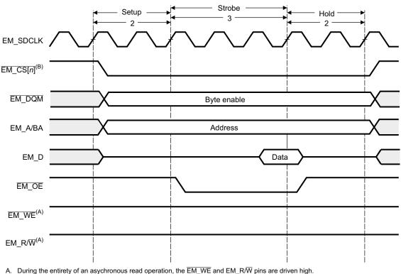
Figure 4-10. Timing Waveform of an Asynchronous Read Cycle in Normal Mode
