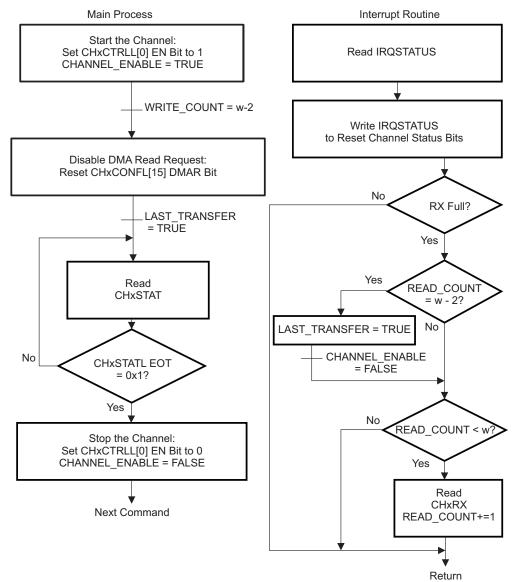
Figure 9-30. Receive-Only With DMA (Master Turbo)
