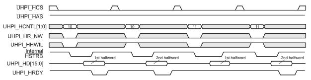
Figure 16-13 shows autoincrement UHPID write cycles when the write FIFO is empty prior to the UHPIA write. The host writes the memory address while UHPI\_HCNTL[1:0] = 10b and writes the data while UHPI\_HCNTL[1:0] = 01b. UHPI\_HRDY does not go low during any of the UHPID write cycles until the FIFO is full.
