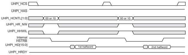
Figure 16-9 includes an UHPID read cycle without autoincrementing. The host writes the memory address during the UHPIA (UHPI\_HCNTL[1:0] = 10b) write cycle, and the host reads the data during the UHPID (UHPI\_HCNTL[1:0] = 11b) read cycle. UHPI\_HRDY goes low for each UHPIA halfword access, but UHPI\_HRDY goes low for only the first halfword access in each UHPID read cycle.
