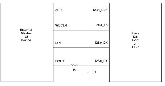
Figure 7-6. Delaying I2S Frame Clock to Overcome Synchronization Problems
