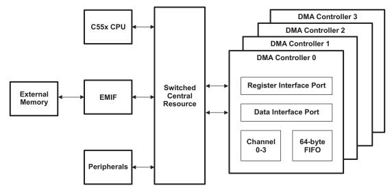
Figure 3-1. Conceptual Block Diagram of the DMA Controller
