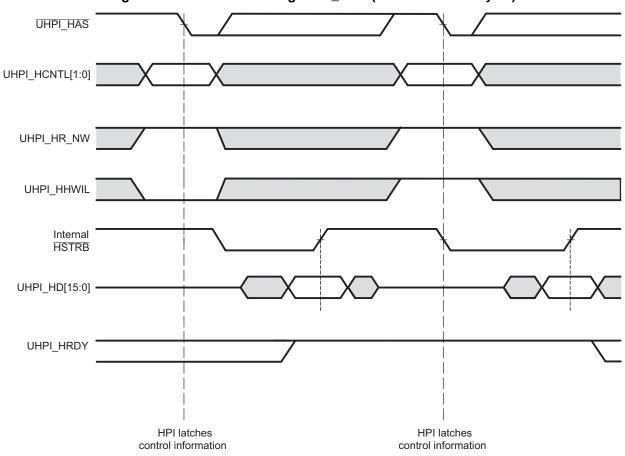
Figure 16-3. Host Read Using UHPI\_HAS (Dual Half-Word Cycle)
