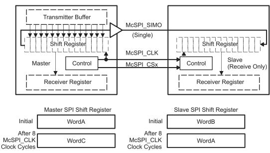
Figure 9-16. McSPI Half-Duplex Transmission (Receive-Only Slave)
