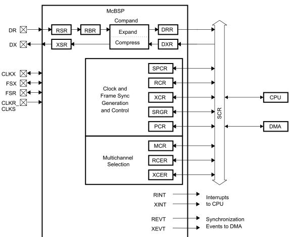
Figure 8-1. McBSP Block Diagram
