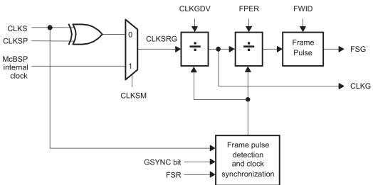
Figure 8-5. Sample Rate Generator Block Diagram
