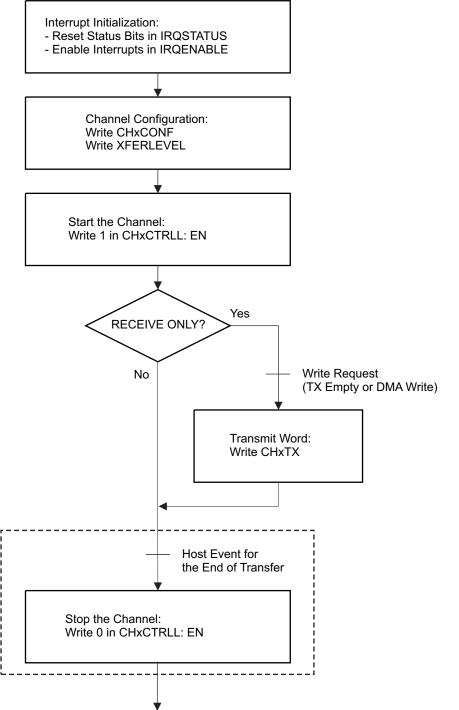
Figure 9-33. FIFO Mode Common Transfer Sequence/Main Process (Master)
