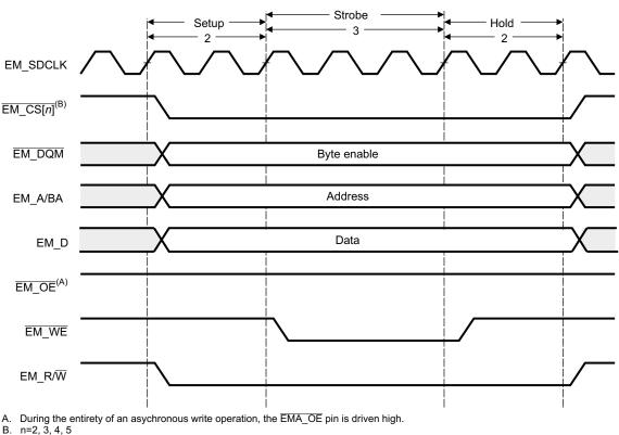
Figure 4-11. Timing Waveform of an Asynchronous Write Cycle in Normal Mode
