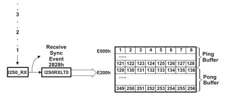
Figure 3-13. Servicing Incoming I2S Data Example DMA Configuration
