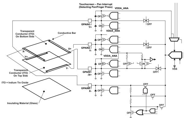
The DSP should be configured to allow SAR interrupts. When the touch screen is not pressed, a pullup resistor biases the PENIRQ buffer high so that an interrupt is not generated. When the touch screen is pressed it creates a path to ground that is lower impedance than the pullup resistor. Therefore, the PENIRQ buffer generates an interrupt and the DSP can then take the steps necessary to digitize the X & Y coordinates.
