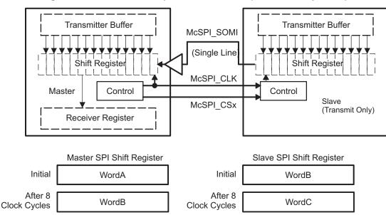
Figure 9-15. McSPI Half-Duplex Transmission (Transmit-Only Slave)
