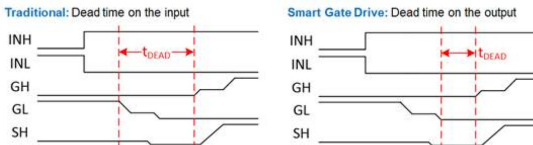
Figure 3. Traditional Dead Time Compared to Smart Gate Drive Dead Time
