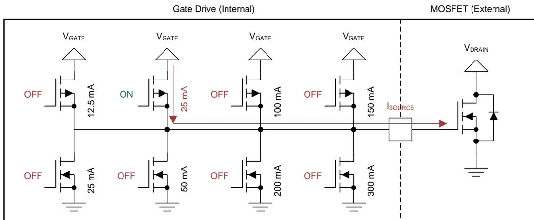
Figure 2. IDRIVE Settings, Programmable Slew Rates
