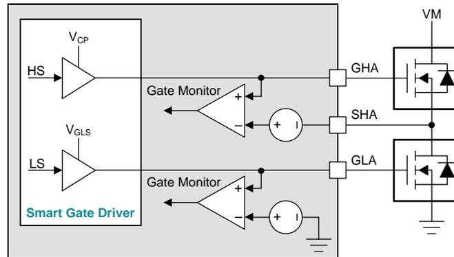
**Figure 4. Smart Gate Drive Gate Monitor**
