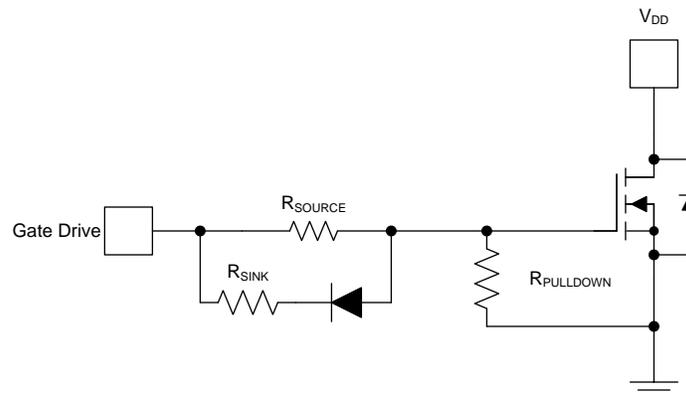
**Figure 1. Traditional Components Between Gate Driver and MOSFET**
