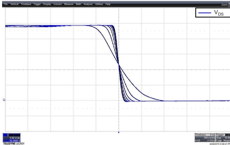
**Figure 2-4.  $V_{DS}$  Persistence Plot Across  $I_{DRIVE}$  Settings**
