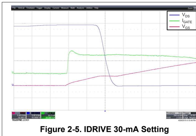
**Figure 2-5.  $I_{DRIVE}$  30-mA Setting**
