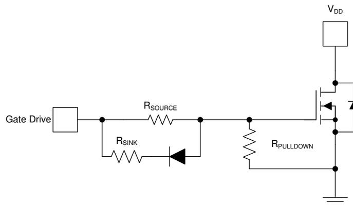
Figure 2-30. Typical Gate Driver Slew Rate External Components
