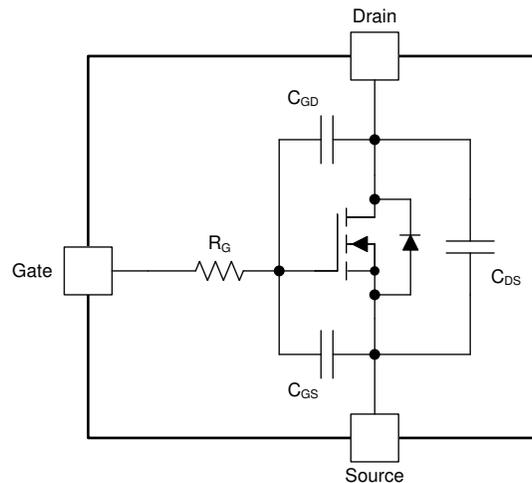
Figure 1-2. MOSFET Circuit Model
