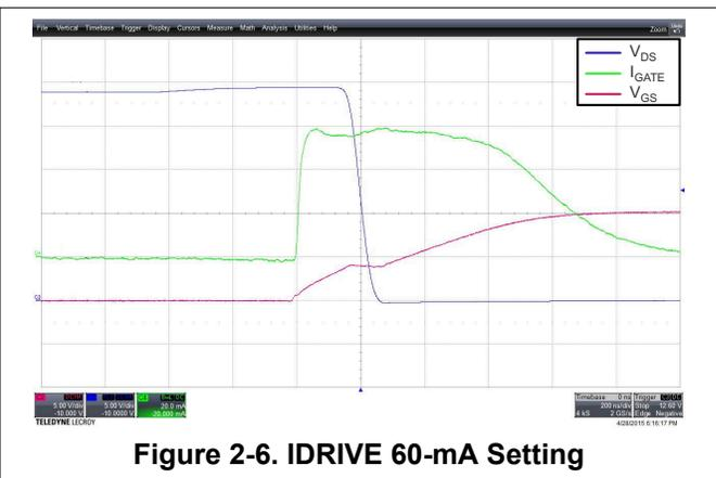
**Figure 2-6.  $I_{DRIVE}$  60-mA Setting**
