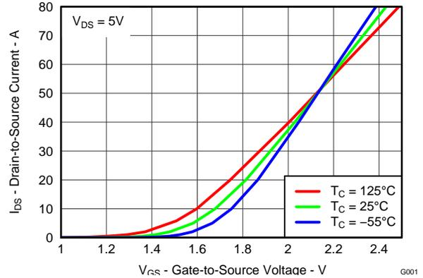
**Figure 3. Transfer Characteristics**
