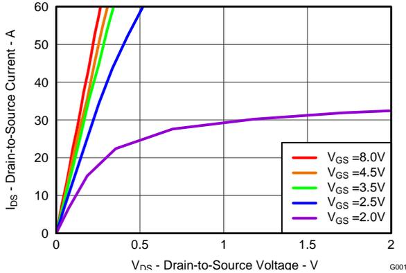
**Figure 2. Saturation Characteristics**
