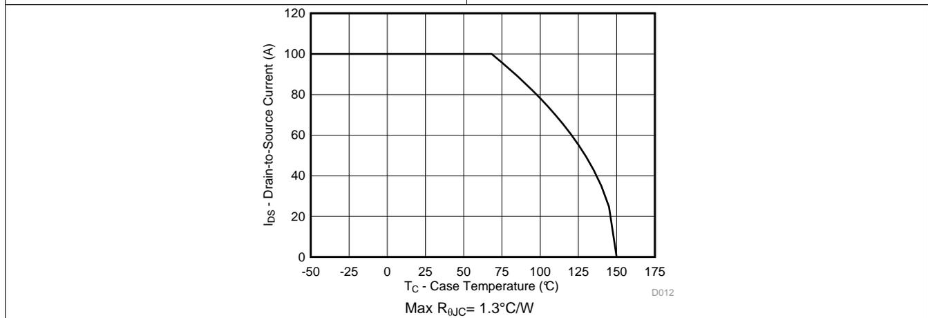
**Figure 12. Maximum Drain Current vs Temperature**
