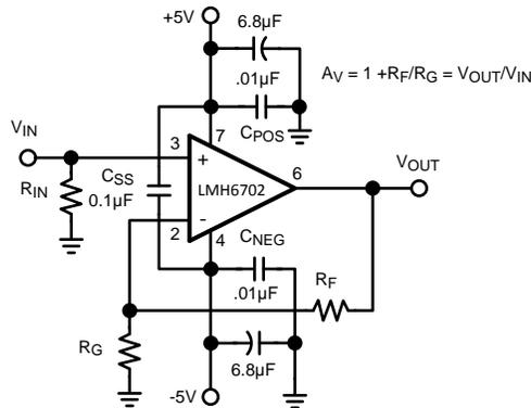
**Figure 21. Recommended Non-Inverting Gain Circuit**
