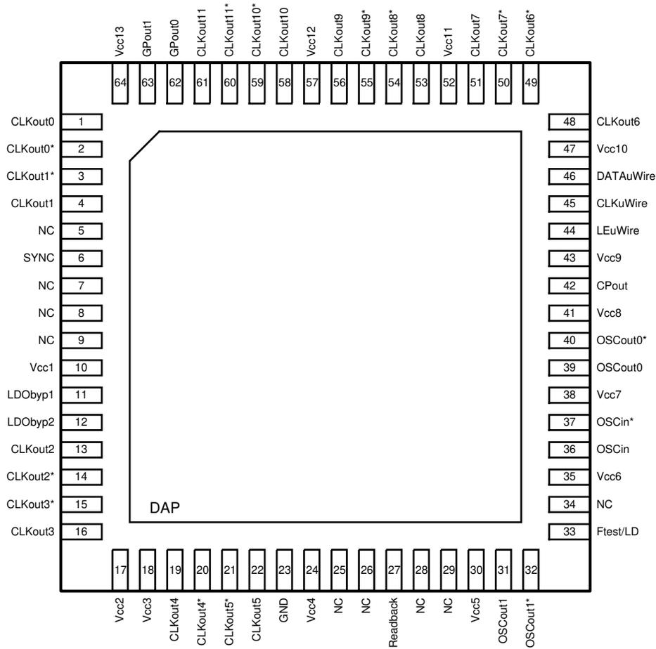
Figure 4-1. NKD Package 64-Pin WQFN Top View
