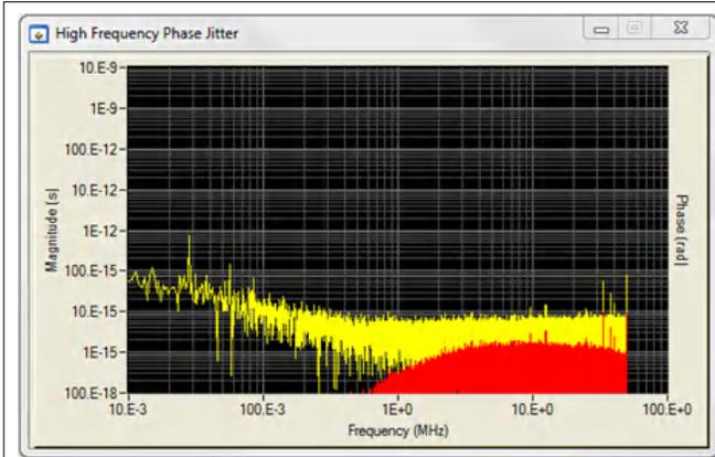
**Figure 8-11. PCIe 3.0 Phase Jitter, 100-MHz HCSL**
