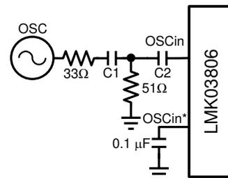
Figure 8-3. 3.3 V<sub>pp</sub> External Reference Interface
