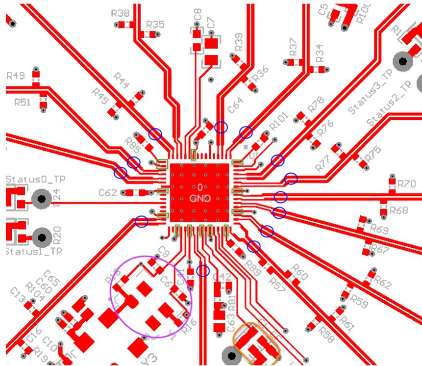
**Figure 8-15. LMK03806 Layout Example**
