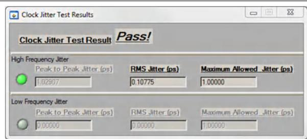
**Figure 8-12. PCIe 3.0 RMS Jitter, 100-MHz HCSL**
