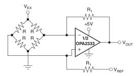
Figure 22. Single Op-Amp Bridge Amplifier
