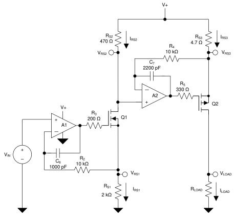
Figure 20. High-Side Voltage-to-Current (V-I) Converter
