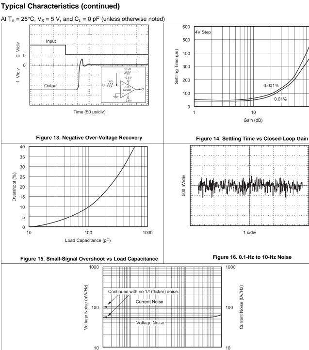
Figure 17. Current and Voltage Spectral Density vs Frequency
