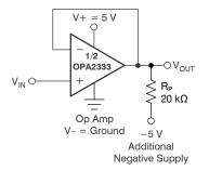
Figure 19. V<sub>OUT</sub> Range to Ground
