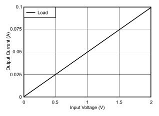
Figure 21. Measured Transfer Function for High-Side V-I Converter
