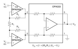
Figure 25. Precision Instrumentation Amplifier
