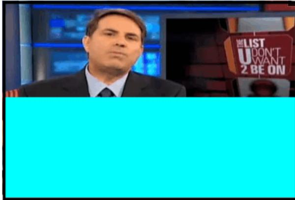
The subpicture feature is enabled when the *SPEN* control bit in the **LCD Raster Subpanel Display n (LCDRASTRSUBPn)** register is set to 1. The *HOLS* bit, when programmed to 0, puts the Default Pixel Data lines at the top of the screen and the active video lines at the bottom of the screen. When the *HOLS* bit is set to 1, Active video lines are at the top of the screen and Default Pixel Data lines are at the bottom of the screen. The *HOLS* bit behavior is shown in Figure 22-15 on page 1692.
