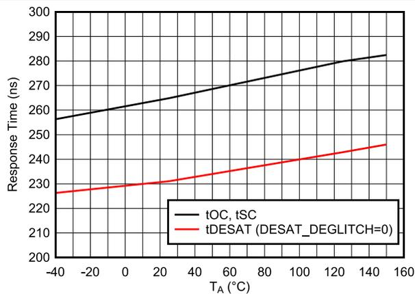
Figure 6-17. Overcurrent Protection Response Time vs. Temperature
