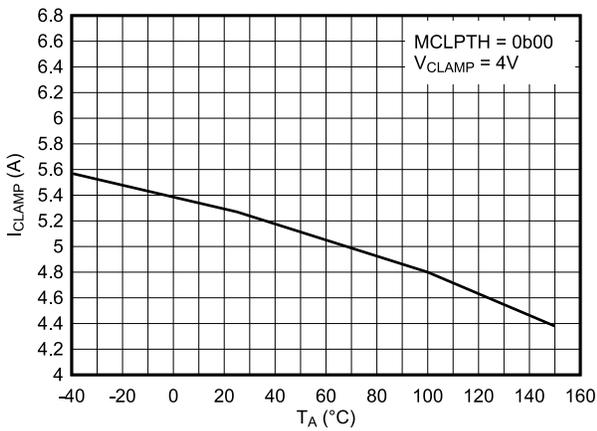
Figure 6-3. Internal Miller Clamp Current vs. Temperature
