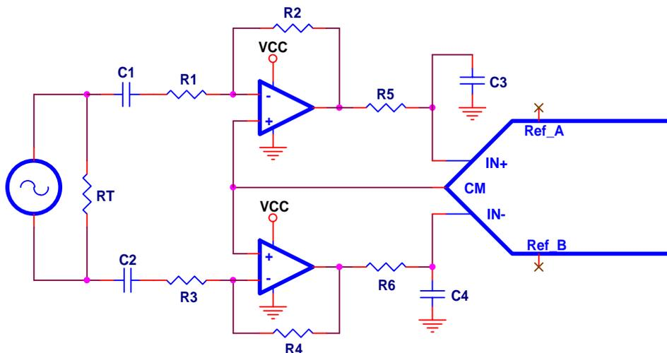
**Figure 22. Differential Output, Differential Input, AC-Coupled, Single Supply**
