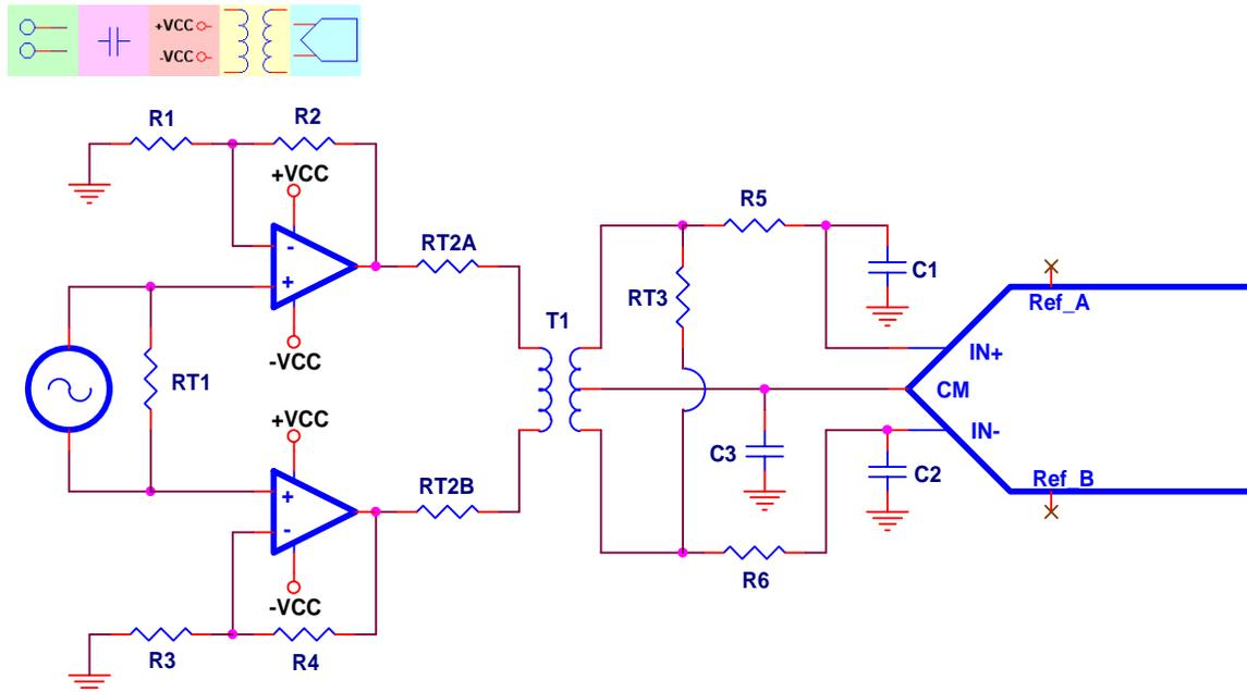
**Figure 31. Differential Input, AC-Coupled, Dual Supply**
