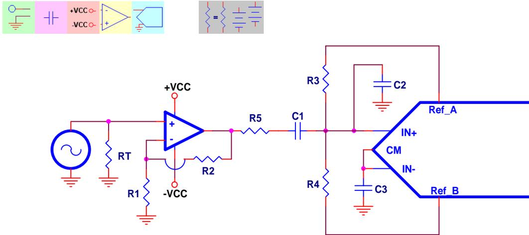
**Figure 13. Single-Ended Output, Single-Ended Input, AC-Coupled, Dual Supply**
