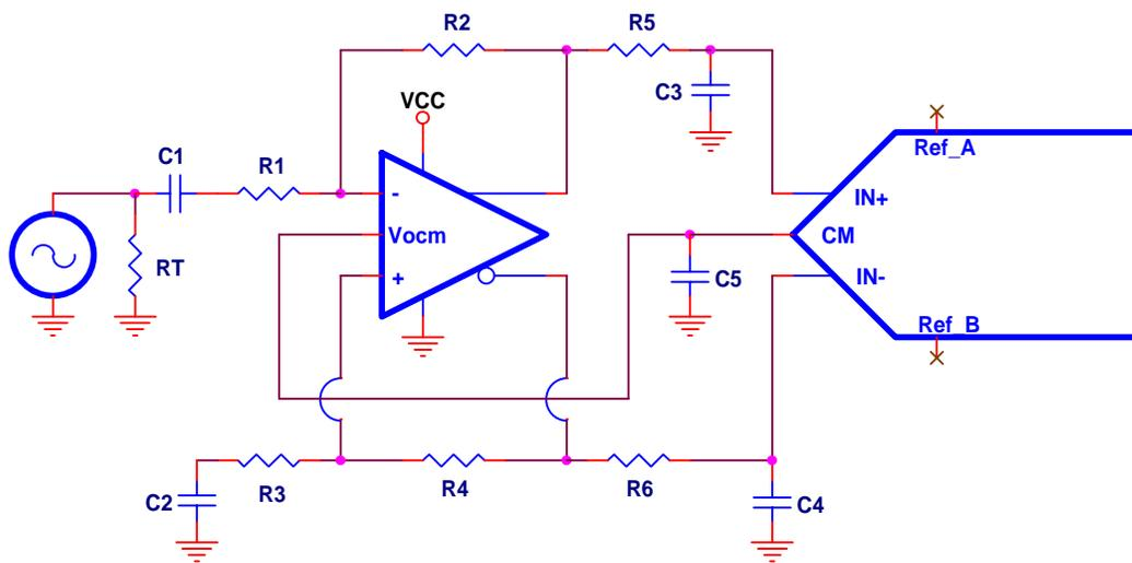
**Figure 3. Single-Ended Input, AC-Coupled, Single Supply**
