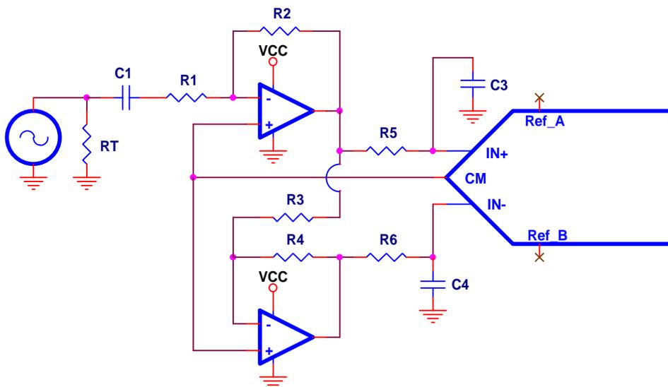
**Figure 18. Alternative Differential Output, Single-Ended Input, AC-Coupled, Single Supply**
