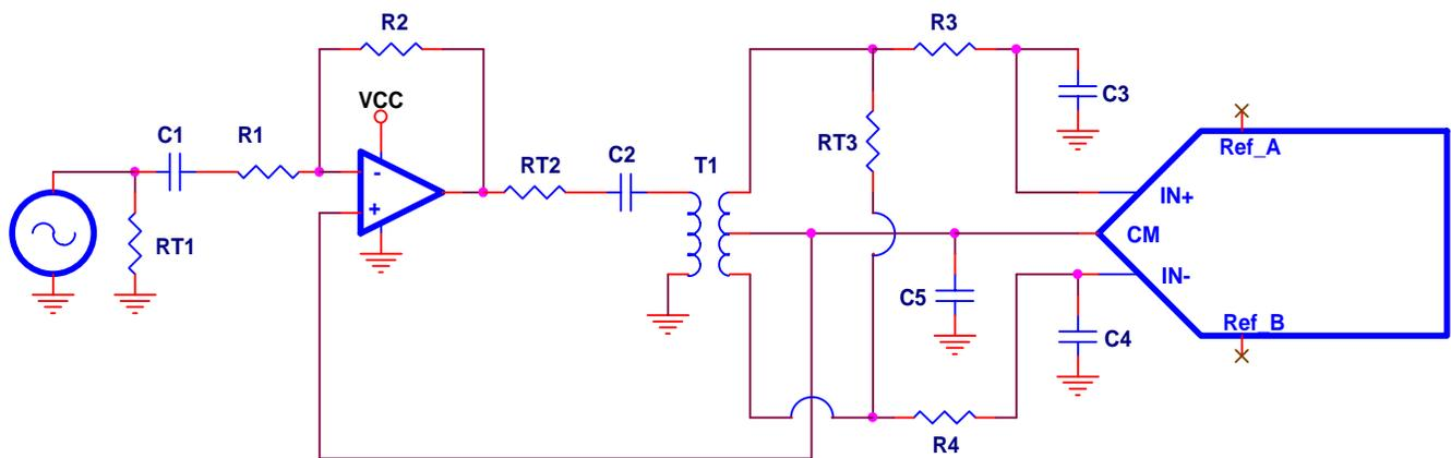
**Figure 25. Single Ended Input, AC-Coupled, Single Supply**
