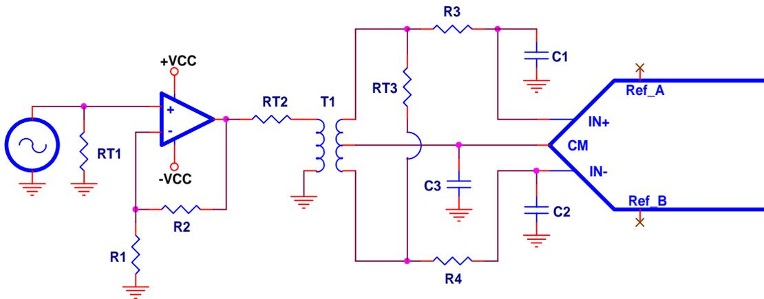
**Figure 28. Single Ended Input, AC-Coupled, Dual Supply**
