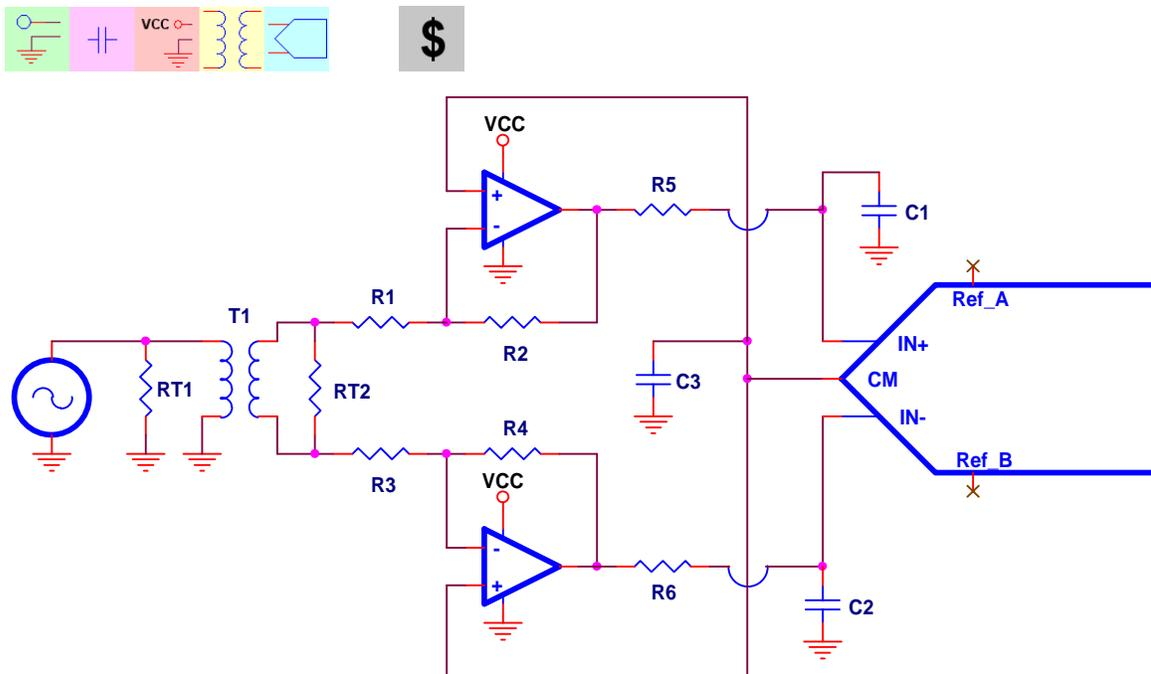
**Figure 27. Transformer Coupled, Buffer on the Secondary Side**
