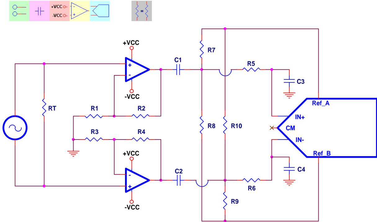
**Figure 23. Differential Output, Differential Input, AC-Coupled, Dual Supply**
