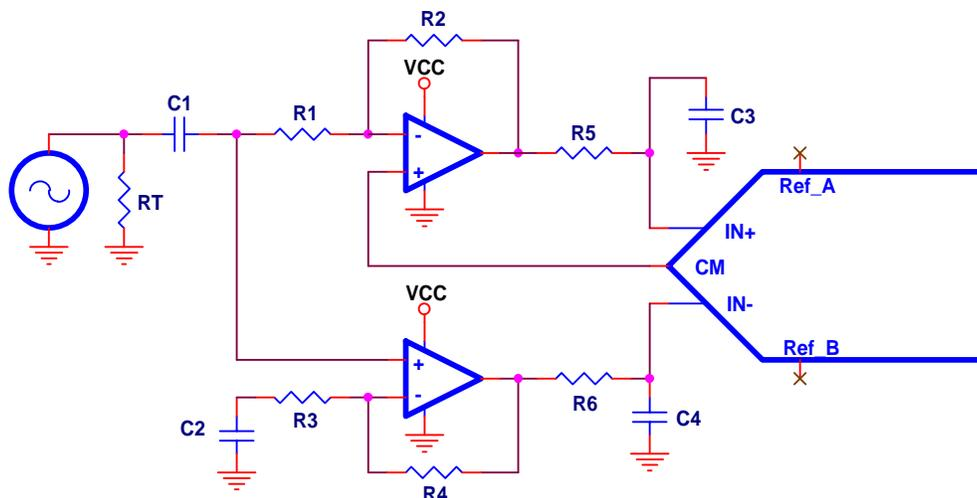
**Figure 17. Differential Output, Single-Ended Input, AC-Coupled, Single Supply**
