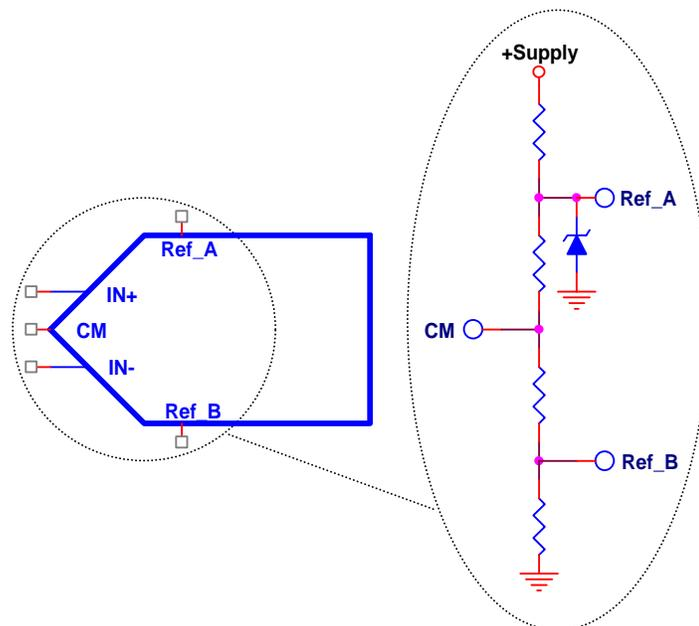
**Figure 2. Reference Structure of Common ADCs**
