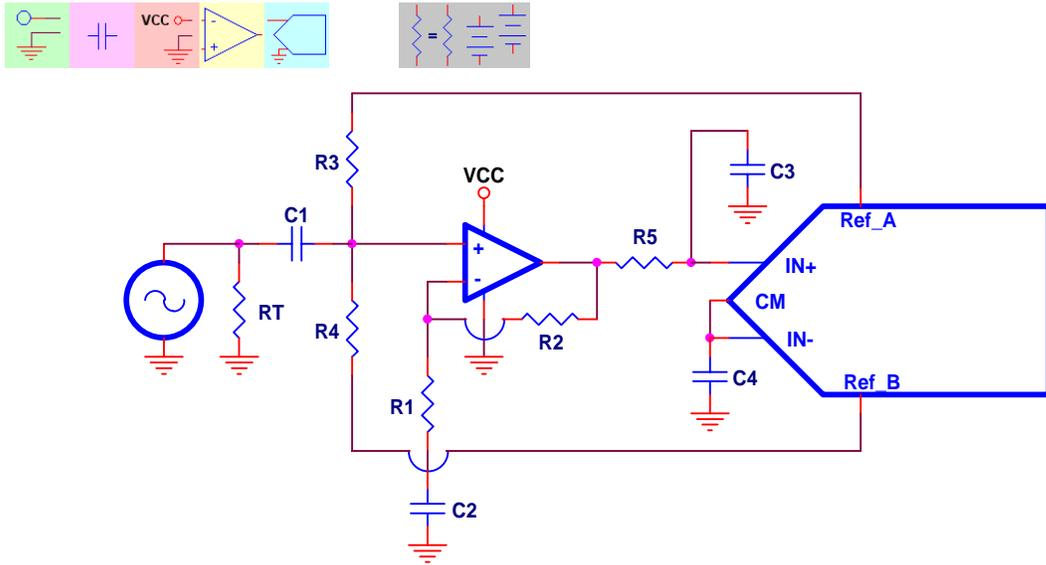
**Figure 11. Single-Ended Output, Single-Ended Input, AC-Coupled, Single Supply**
