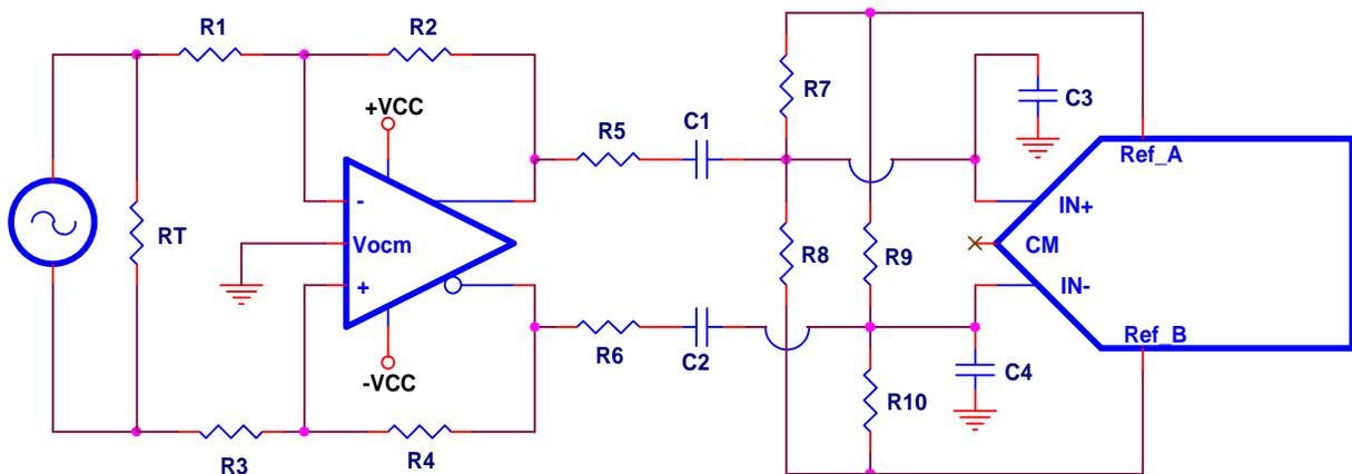
**Figure 7. Differential Input, AC-Coupled, Dual Supply**
