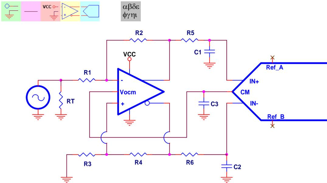
**Figure 5. Single-Ended Input, DC-Coupled, Single Supply**
