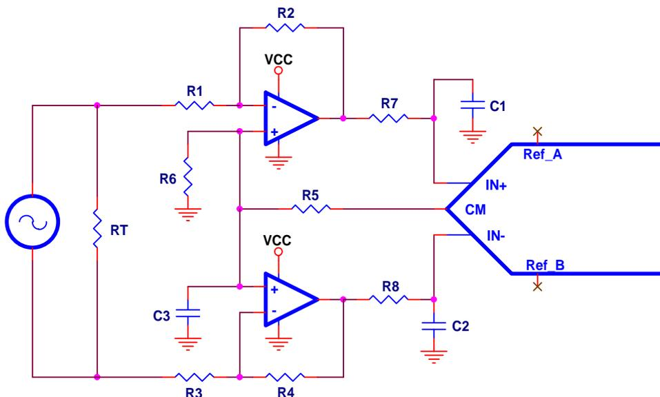
**Figure 24. Differential Output, Differential Input, DC-Coupled, Single Supply**
