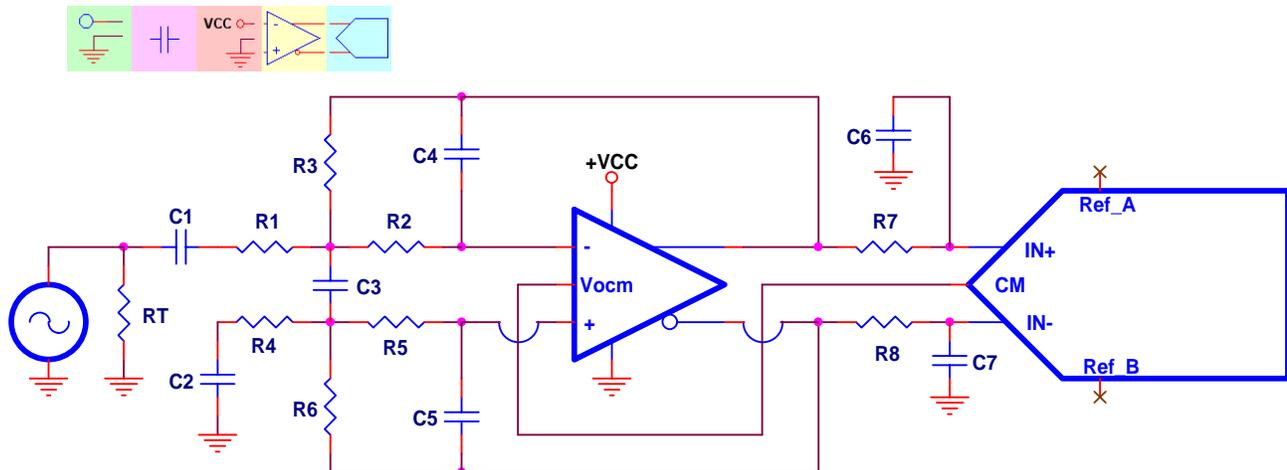
**Figure 10. Antialias Filter Using a Fully Differential Op Amp**
