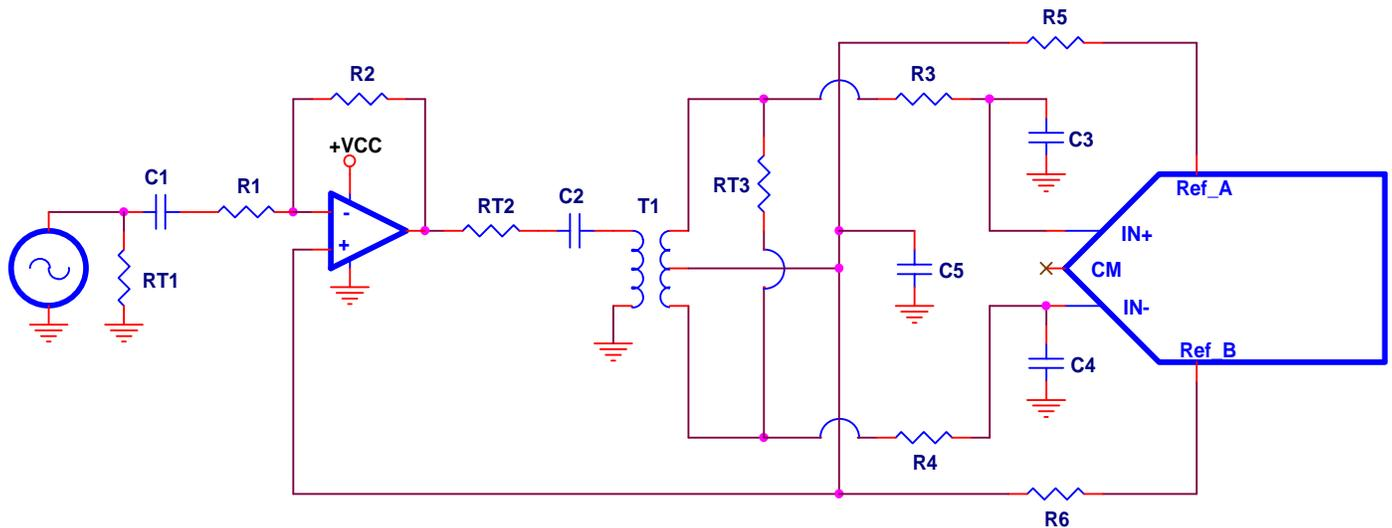
**Figure 26. Transformer Coupled, Pre-Transformer, Derived Reference**
