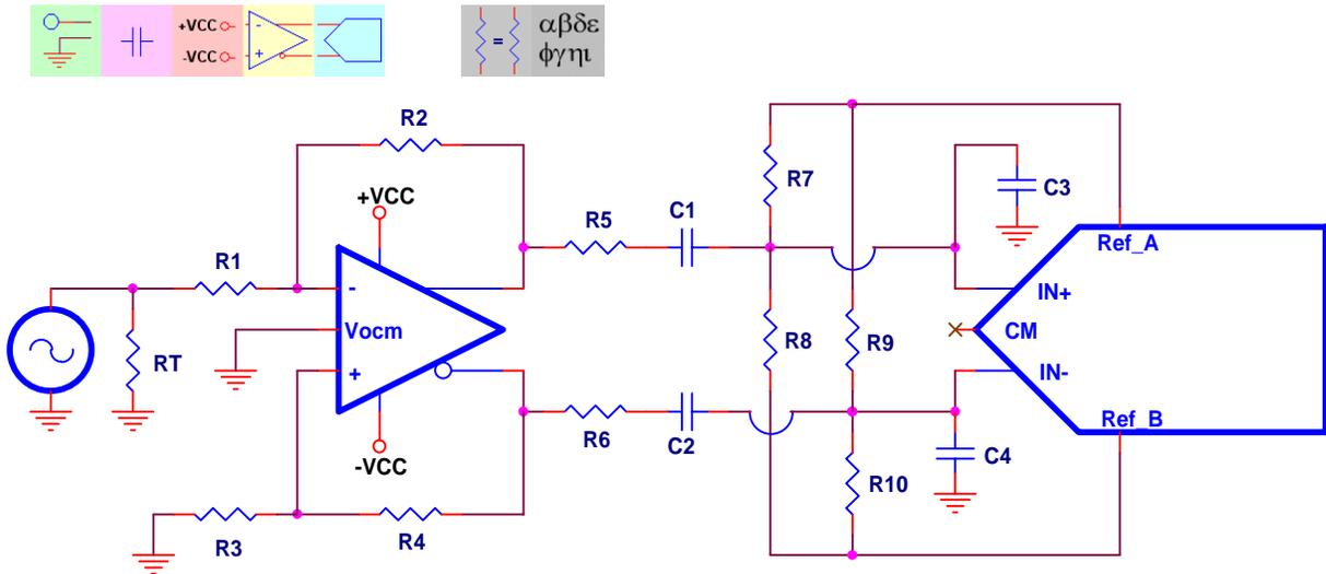
**Figure 4. Single Ended Input, AC-Coupled, Dual Supply**
