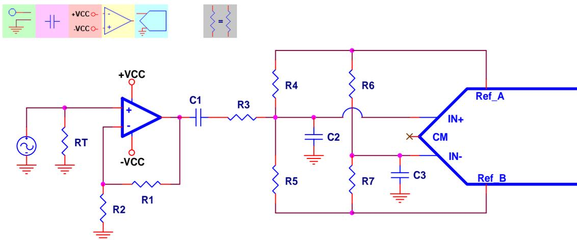
**Figure 14. Single-Ended Output, Single-Ended Input, AC-Coupled, Dual Supply**
