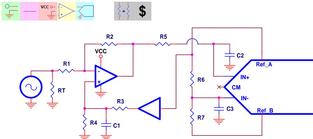
**Figure 16. Single-Ended Output, Single-Ended Input, DC-Coupled, Single-Supply**
