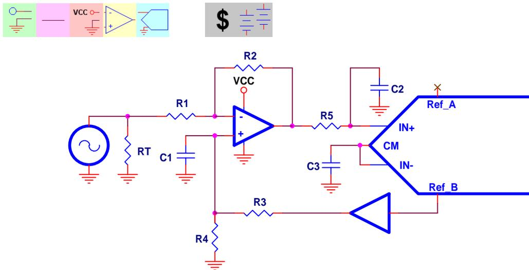
**Figure 15. Single-Ended Output, Single Ended Input, DC Coupled, Single Supply**
