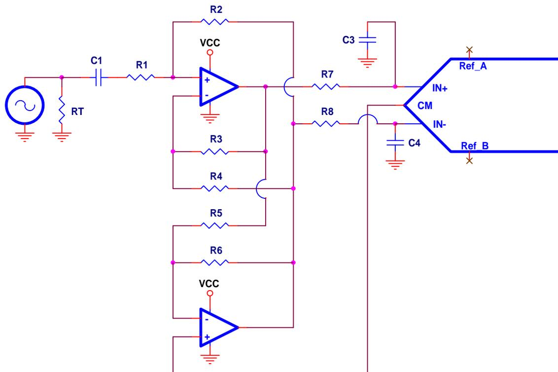
**Figure 19. Alternative Differential Output, Single-Ended Input, AC-Coupled, Single Supply**
