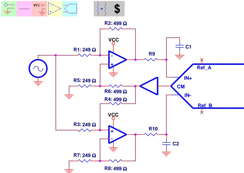
**Figure 21. Differential Output, Single-Ended Input, DC-Coupled, Single Supply**
