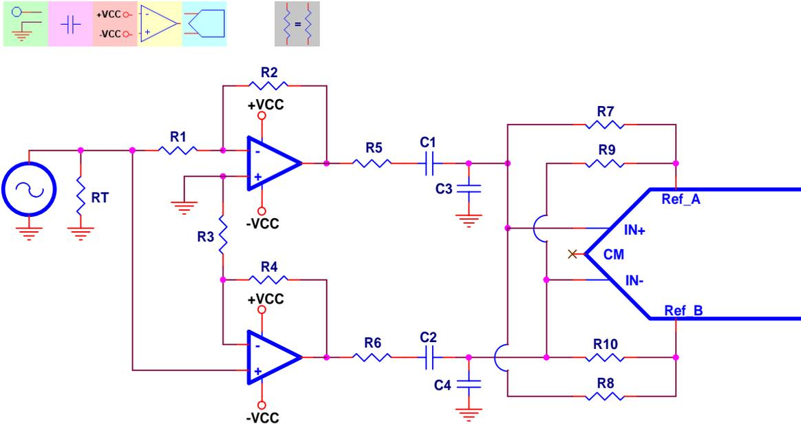
**Figure 20. Differential Output, Single-Ended Input, AC-Coupled, Dual Supply**
