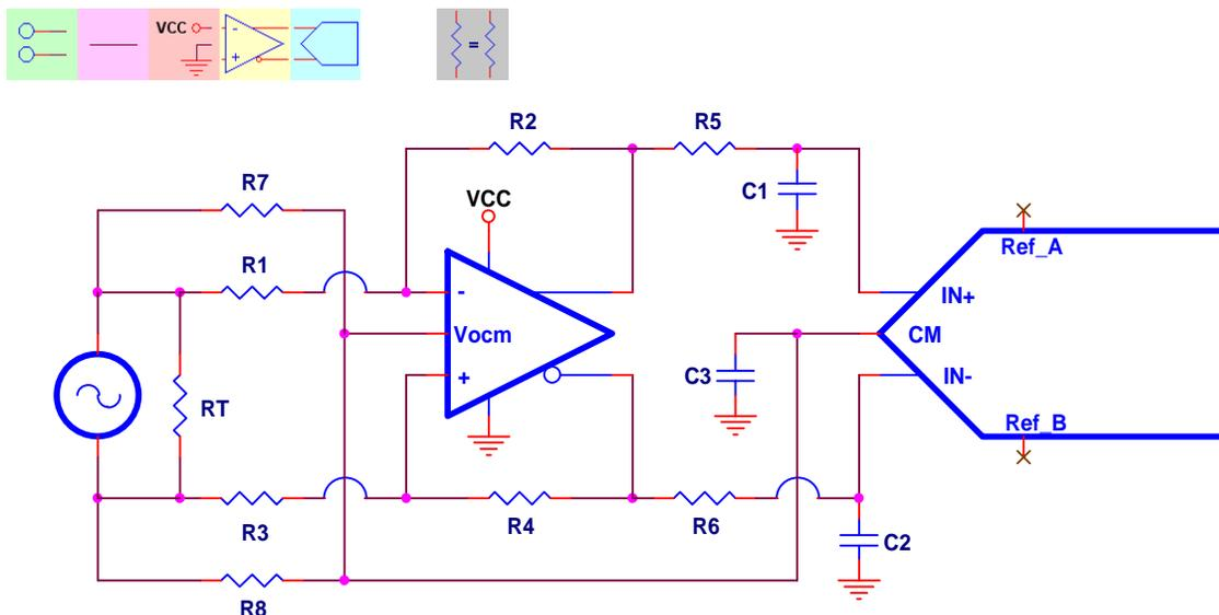
**Figure 8. Differential Input, DC-Coupled, Single Supply—Common Mode From Source**
