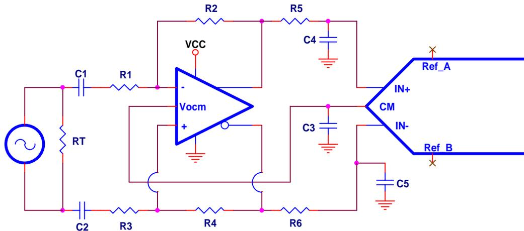
**Figure 6. Differential Input, AC-Coupled, Single Supply**
