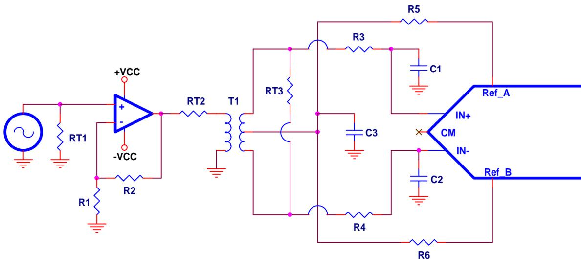
**Figure 29. Single-Ended Input, AC-Coupled, Dual Supply**
