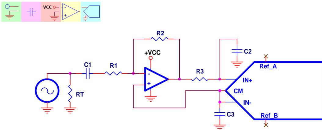
**Figure 12. Single-Ended Output, Single-Ended Input, AC-Coupled, Single Supply**
