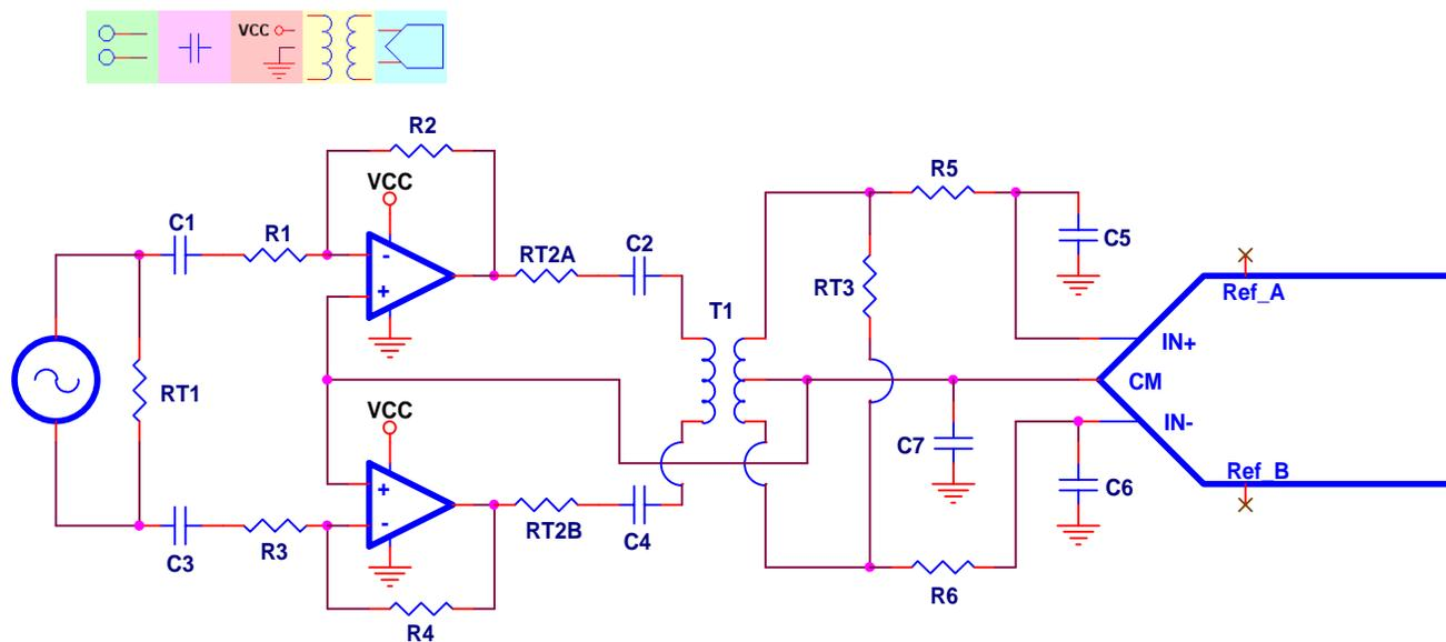
**Figure 30. Differential Input, AC-Coupled, Single Supply**
